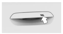
Touch the grooved surface on the external door handle of a closed front door with your finger and hold it there without grasping the recessed arip.
