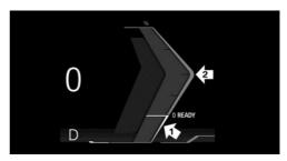
Needle in range of arrow 1: display for energy recovery such as while decelerating CHARGE.
