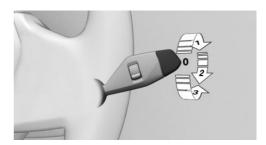
Turn the outer switch upward.
