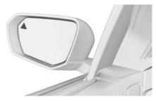
The light in the exterior mirror warns of a possible collision.
