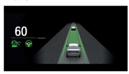
An example of active Driver Assistance: indicator and warning lights for Distance Control and Assisted Driving are displayed. At the same time, the Distance Control is animated in Assisted View.
