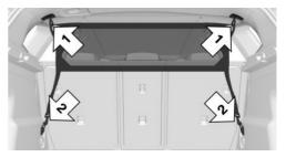
4. Use the two lower hooks to hook the cargo area partition net into the lashing eyes in the cargo area, arrow 2.
