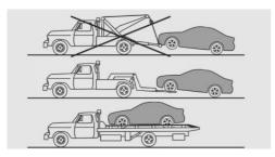
Your vehicle should be transported with a tow truck with a so-called spectacle lift or on a loading platform.
