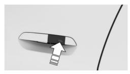
Hold the near field communication antenna of the smartphone directly and centered on the external door handle of the driver's door. The position of the near field communication antenna depends on the smartphone model.
