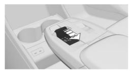
Pull the selector lever from selector lever position D to D/I.
