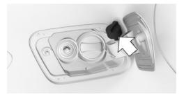
4. Using the filler nozzle, add at least the recommended top-up quantity.
