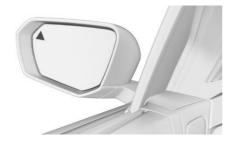
The light in the exterior mirror warns of a possible collision.
