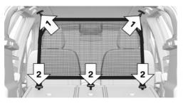
4. Attach the cargo area partition net with the lower three hooks into the three front loops on the folded down rear seat backrest, arrows 2. You may need to lift the rear seat backrests slightly in order to do this.
