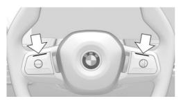
Depending on the equipment, the two LEDs above the keypads illuminate analog to the displays in the instrument cluster.
