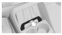
The retaining clip can be opened to make it easier to insert and remove a mobile phone.
