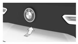
▶ Unlock the vehicle and then press the button on the outer side of the cargo area.
