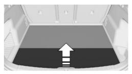
Hold the edge of the cargo area floor and fold it forward.
