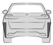
The radar sensors are located on the side in the rear bumper.
