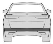
The ultrasonic sensors of the parking assistance systems are located in the rear bumper.
