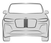
The front radar sensor is located in the radiator arille.
