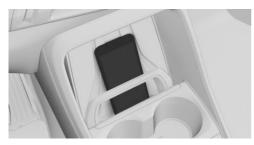
Insert the mobile phone upright and in the center behind the retaining clip and slide it down to the stop. The mobile phone display must point upwards.
