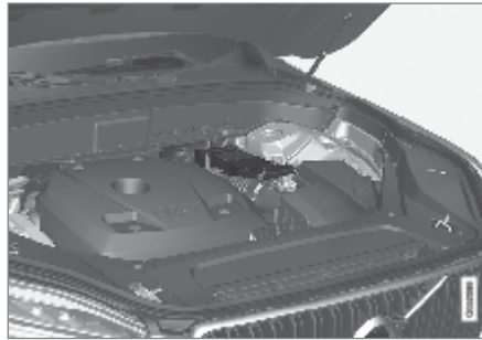
The 12 V support battery is located in the engine compartment.
