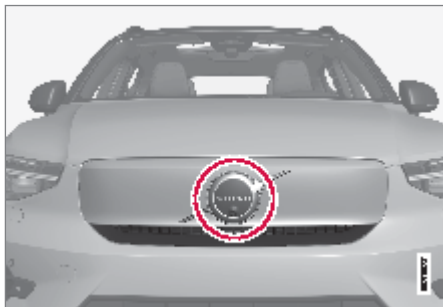
Location of the front radar sensor
