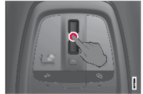
Ventilation position, rear edge raised.
