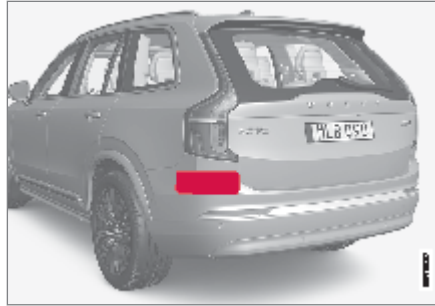
Location of rear radar sensors
