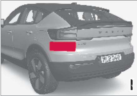
Location of rear radar sensors
