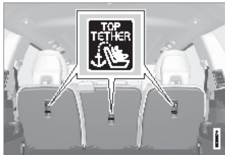
Five-seat and seven-seat models: Top tether anchors and symbols on the rear side of the second row
