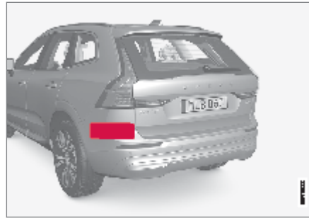
Location of rear radar sensors
