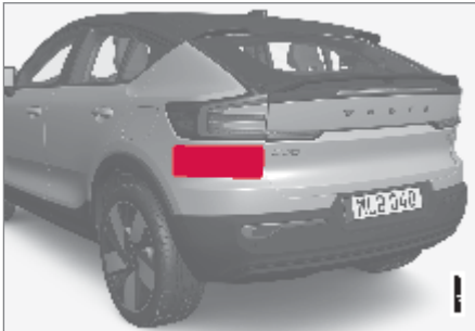
Location of rear radar sensors
