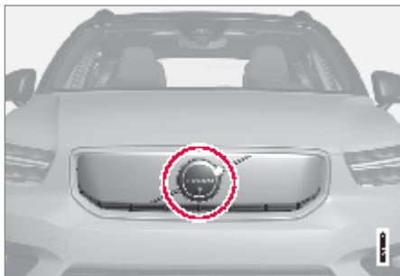
Location of the front radar sensor
