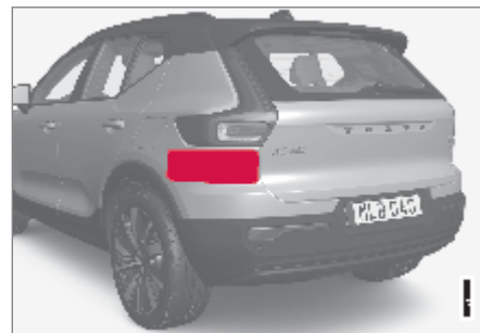
Location of rear radar sensors
