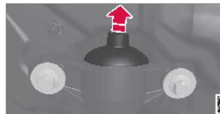
The rubber cap is located above the adjustment knob.
