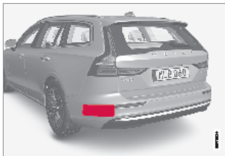
Location of rear radar sensors
