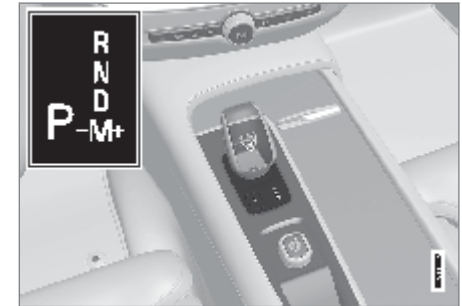
Overview of gear selector and gear shift pattern in the instrument panel.
