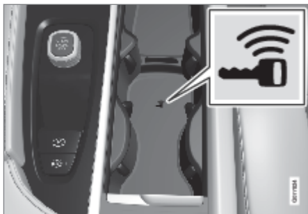
Location of the backup reader in the tunnel console.
