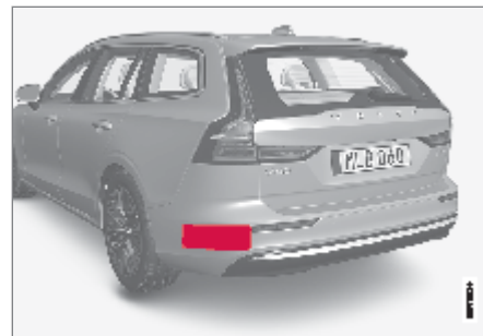
Location of rear radar sensors
