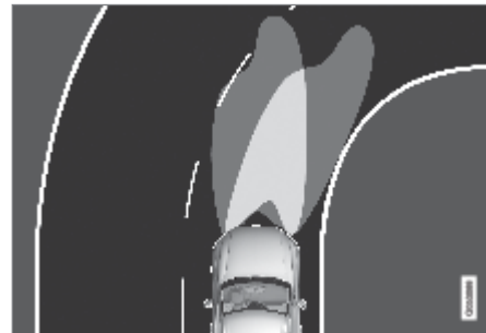
Headlight pattern without Active Bending Lights (left), and with (right).
