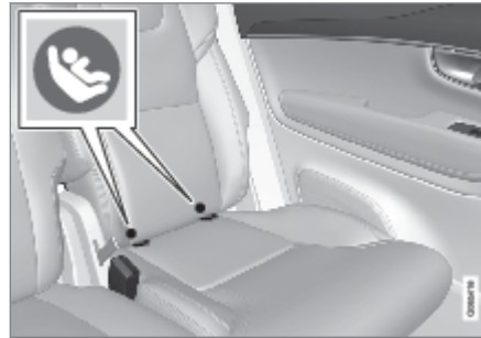
Location of the ISOFIX/LATCH anchors
