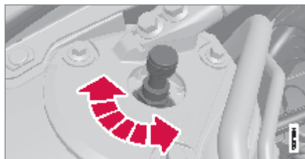
The rubber cap is located above the adjustment knob.
