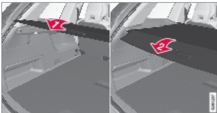
The rear flap mounted on the inside of the tailgate supplements the cargo compartment cover.
