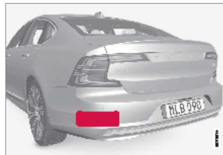
Location of rear radar sensors
