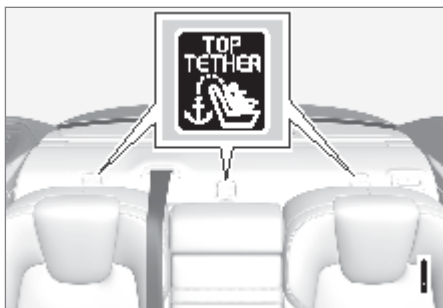
Top tether anchors and symbols on the rear parcel shelf.
