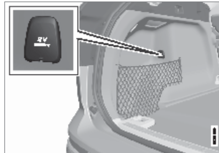
12 V outlet in the cargo compartment*.
