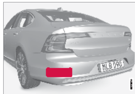
Location of rear radar sensors
