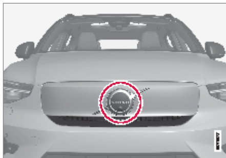
Location of the front radar sensor
