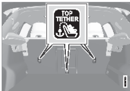
Top tether anchors and symbols on the rear side of the rear seat backrests.
