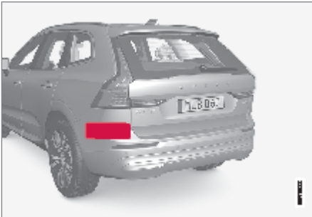
Location of rear radar sensors
