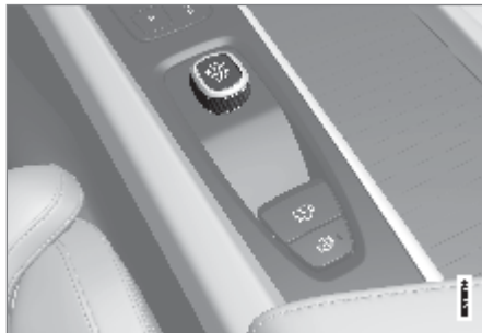
Start knob in the tunnel console.
