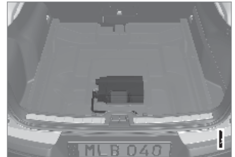
Mild hybrid vehicles have a 48 V support battery under the cargo compartment. The battery may only be handled by authorized workshop personnel.
