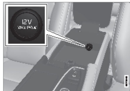
12 V outlet in the tunnel console, front seat.
