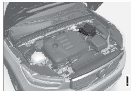
The start battery is located in the engine compartment.
