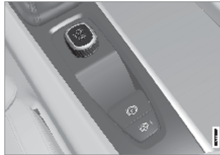
Start knob in the tunnel console.
