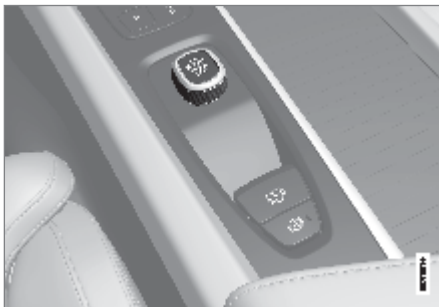
Start knob in the tunnel console.
