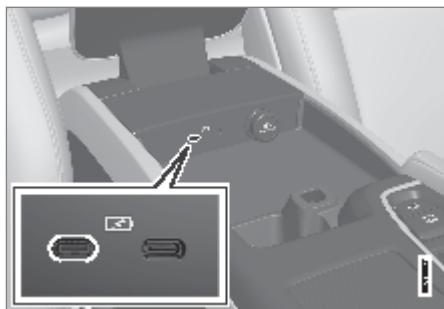
USB ports (type C), front seat.
