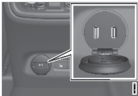
USB ports (type C) in tunnel console, rear seat.
