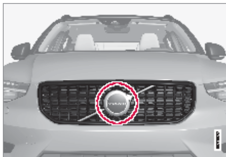
Location of the front radar sensor
