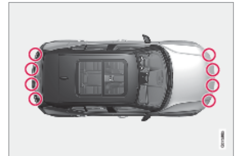
Location of the parking sensors around the vehicle
