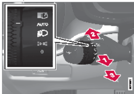
Steering wheel lever with lighting ring.
