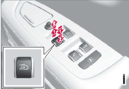
Sun curtain control.
