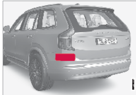
Location of rear radar sensors
