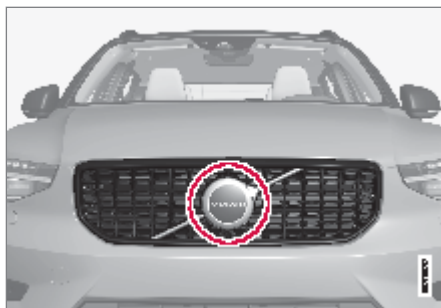
Location of the front radar sensor
