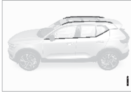
Components that should be washed with a cleaning product with a pH value between 3.5 and 11.5.
