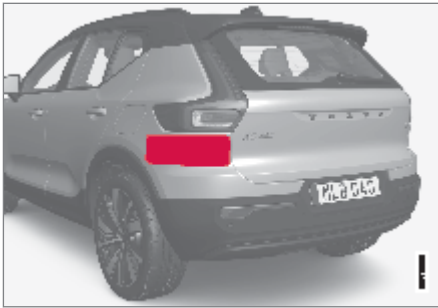
Location of rear radar sensors
