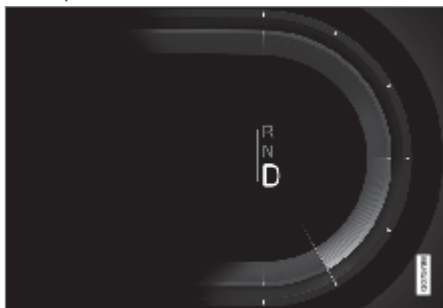
Indication in the instrument panel during regenerative braking.
