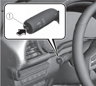
1. High beam control switch
