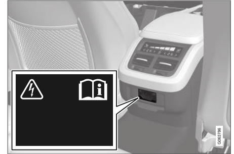
Electrical socket in the tunnel console, rear seat.
