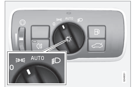
Knob for headlamp control in the position for position lamps.
