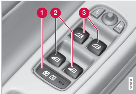
Driver's door control panel.
