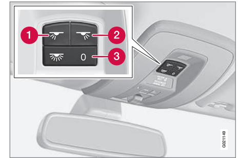
Controls in roof console for the front reading lamps and passenger compartment lighting.
