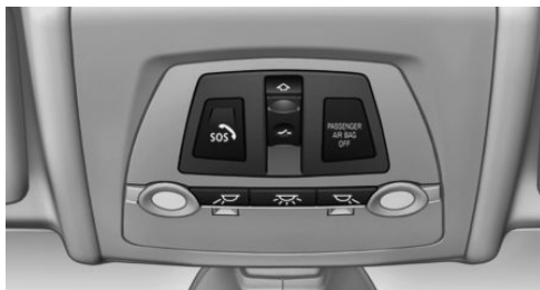
SOS button in the roofliner
