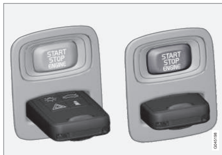
Ignition switch with remote control key extracted/inserted.
