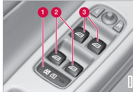
Driver's door control panel.
