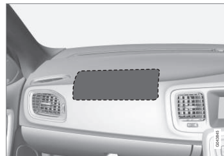
Location of the front passenger airbag in a right-hand drive car.
