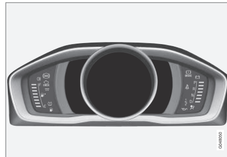
Information display, digital instrument panel*.
