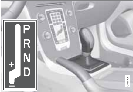
D: Automatic gear positions. +/-: Manual gear positions.
