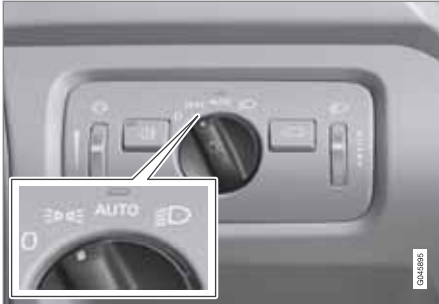
Headlamp control in position for position/parking lamps.
