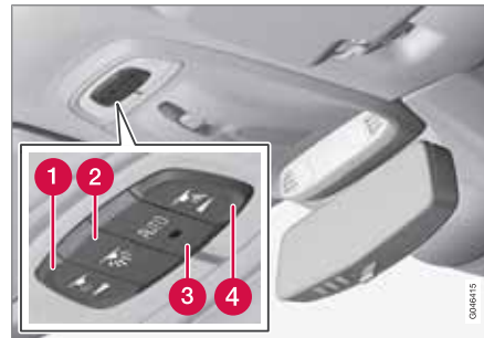
Controls in the roof console for the front reading lamps and ceiling lamps.
