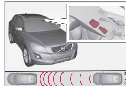
Laser sensor transmitter and receiver window 1 .
