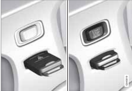
Ignition switch with remote control key extracted/inserted.
