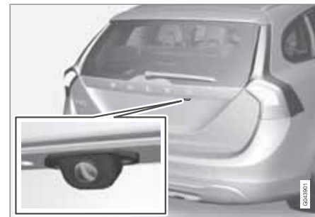
Camera location next to the opening handle.
