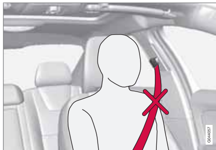
Incorrectly fitted seatbelt. The belt must rest on the shoulder.
