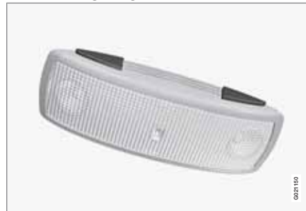
Rear roof lighting.
