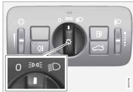
Headlamp control in position for position/parking lamps.
