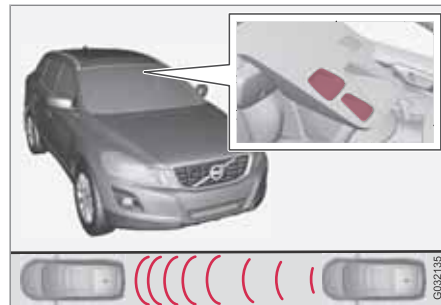
Laser sensor transmitter and receiver window.
