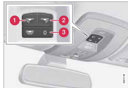
Controls in roof console for the front reading lamps and passenger compartment lighting.
