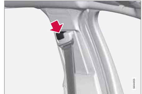
Height adjustment of seatbelt's upper fix-point. Press in the button and move the upper fix-point vertically. Position the upper fix-point as high as possible without the belt chafing against your throat.
