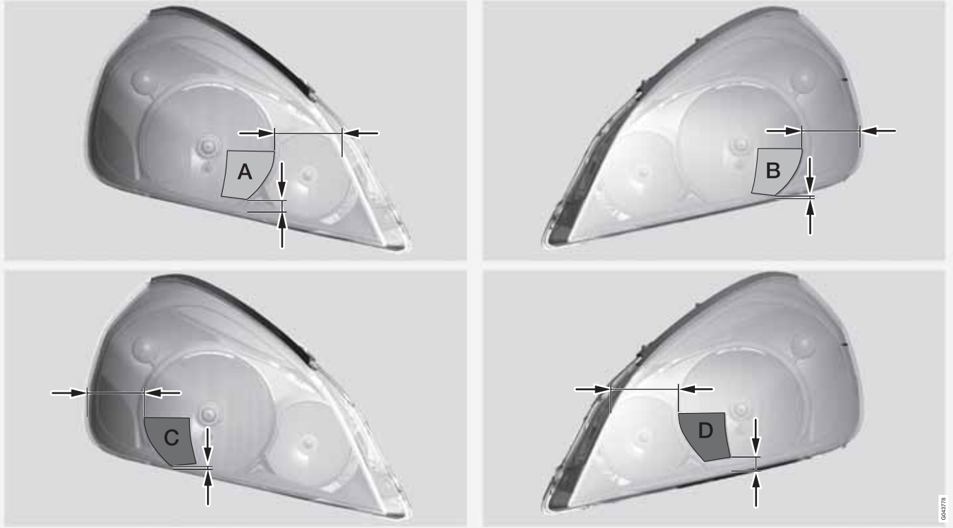
Upper row: masking left-hand drive cars, templates A and B. Lower row: masking right-hand drive cars, templates C and D.
