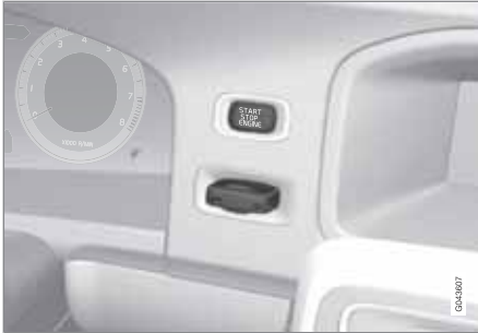
Ignition switch with inserted remote control key and START/STOP ENGINE button.
