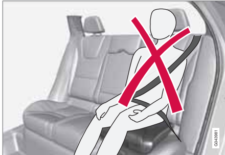
Incorrect position, the head restraint must be adjusted as high as the head and the seatbelt must not be below the shoulder.
