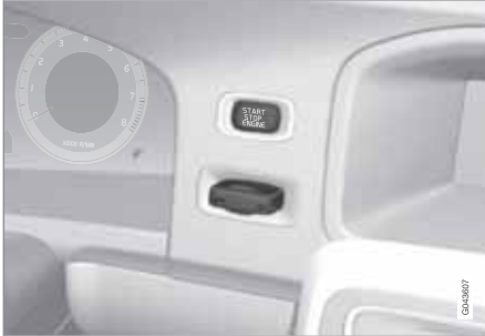
Ignition switch with inserted remote control key.
