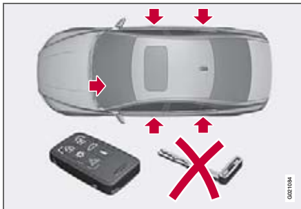
Active locks for remote control key, with privacy locking activated.
