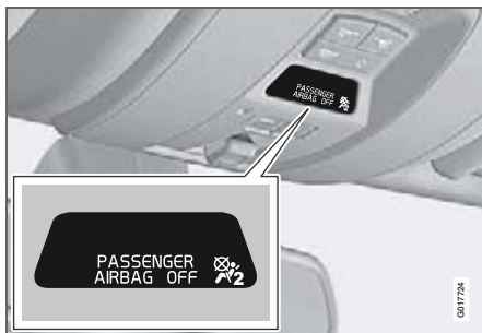
Indicator in the roof console showing that the passenger airbag (SRS) is deactivated.
