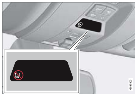
Indicator in roof console showing that the passenger airbag (SRS) is activated.
