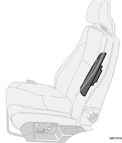
The side impact airbags are installed in the front seat backrest frames
