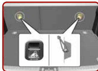
Securing with "Tether Anchorage" system [3]
