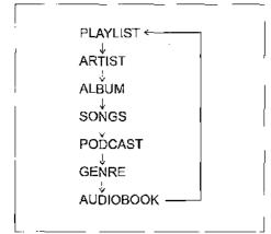
Press "TUNE/FLD PUSH SOUND" knob (2) to select the desired mode.
