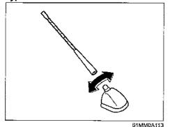
The radio antenna on the roof is removable. To remove the antenna, turn it counterclockwise. To reinstall the antenna, turn it clockwise firmly by hand.
