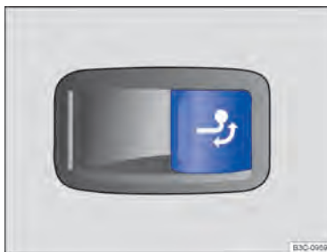
Fig. 136 On the right of the luggage compartment: button for releasing the ball coupling.
