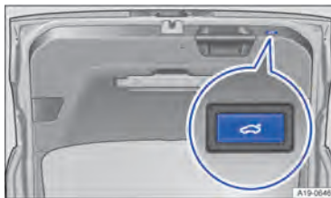
Fig. 68 In the open tailgate: button for closing boot lid electrically.
