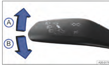
Fig. 85 On the left-hand side of the steering column: turn signal and main beam lever.
