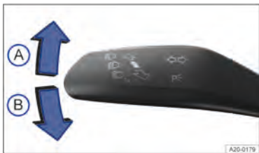
Fig. 88 On the left-hand side of the steering column: turn signal and main beam lever.
