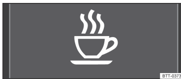
Fig. 15 On the instrument cluster display: Driver Alert System symbol.
