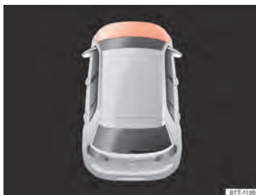
Fig. 177 On the instrument cluster display: the bonnet is open or not closed properly (illustration).
