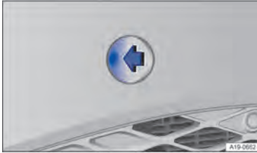
Fig. 169 In the front bumper on the right: removing the cover.
