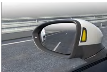
Fig. 113 In the exterior mirror housing: visual displays of the lane change system.
