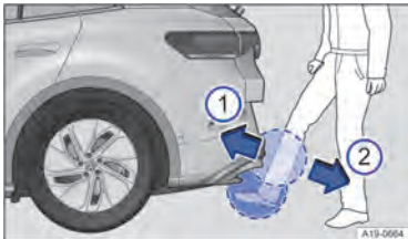
Fig. 70 Boot lid with sensor-controlled closing (Easy Close).
