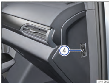
Fig. 9 With open front passenger door (left-hand drive vehicles): key-operated switch in the dash panel (mirrored for right-hand drive vehicles).
