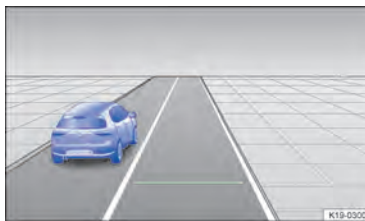
Fig. 103 On the instrument cluster display: slower vehicle detected in the left-hand lane (illustration).
