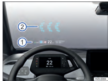
Fig. 14 In the driver's field of vision: head-up display close range ① and AR head-up display ②.
