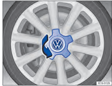
Fig. 188 Removing the centre wheel trim by turning.
