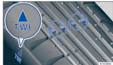
Fig. 185 Tyre tread: tread wear indicators.
