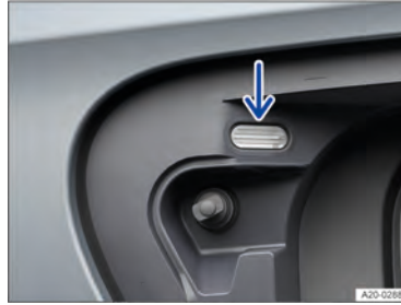
Fig. 148 Behind the charging socket flap: charging process indicator.
