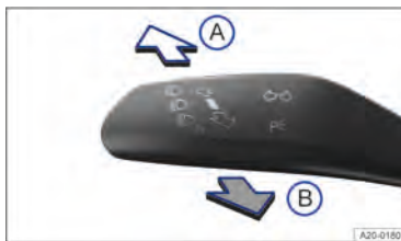
Fig. 87 On the left-hand side of the steering column: turn signal and main beam lever.
