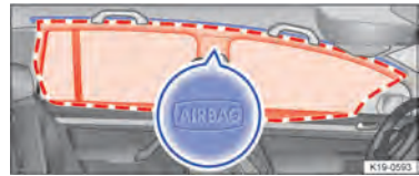
Fig. 38 On the left-hand side of the vehicle: location and deployment zone of the curtain airbag.
