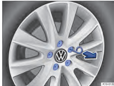
Fig. 190 Removing the wheel bolt caps.
