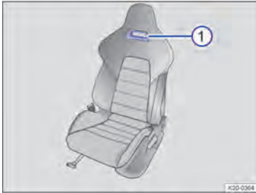
Fig. 49 In the backrest of the Top sports seat on the passenger side: opening for the top tether (schematic diagram).
