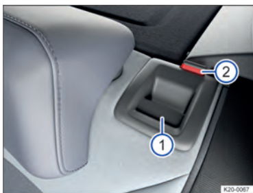
Fig. 77 In the rear seat backrest: release button.
