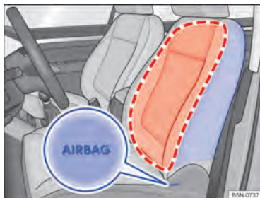
Fig. 37 On the side of the front seat: location and deployment zone of the side airbag.
