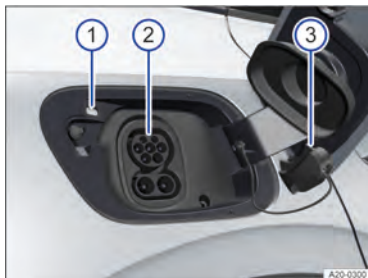
Fig. 147 Behind the charging socket flap at the rear right: charging socket.
