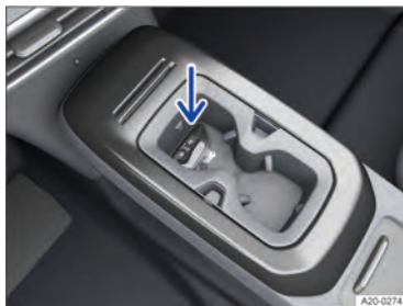
Fig. 99 In the centre console: emergency start function.
