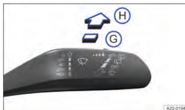
Fig. 92 On the right-hand side of the steering column: operating the rear window wiper.
