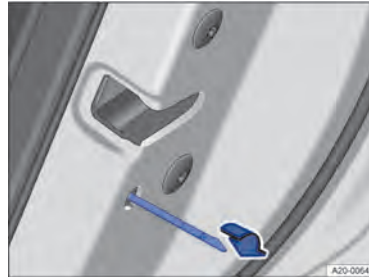
Fig. 62 In the end face of the right-hand door: locking the vehicle manually with the spare key.
