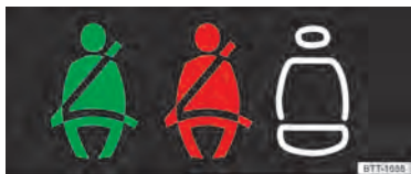
Fig. 20 On the instrument cluster display: seat belt status for the rear seats.
