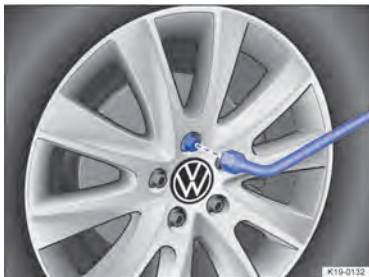
Fig. 196 Wheel change: Unscrew the wheel bolts with the wheel wrench.
