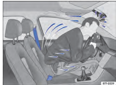
Fig. 23 An unbelted driver is thrown forwards.
