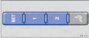
Fig. 83 On the outside of the driver seat: memory buttons.
