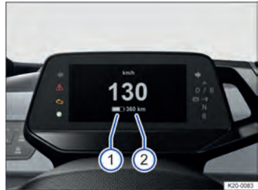
Fig. 11 In the digital instrument cluster: charge level of the high-voltage battery ① and vehicle range ②.
