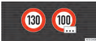
Fig. 16 In the instrument cluster display: example of recognised speed limits with generic additional sign.
