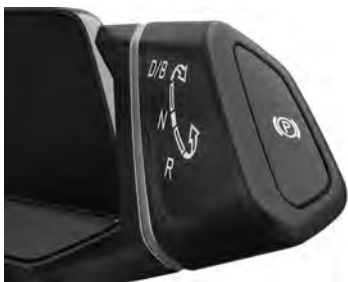
Fig. 114 On the driving mode selector: P button for the electronic parking brake.
