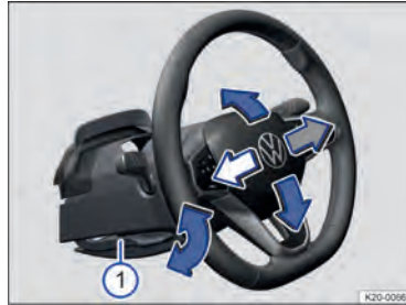
Fig. 72 Below the steering wheel in the steering column trim: lever for mechanical adjustment of the steering wheel position.
