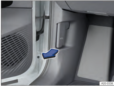
Fig. 173 In the footwell on the driver side: bonnet release lever (schematic diagram).
