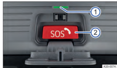
Fig. 52 Control for emergency call: indicator lamp and button.
