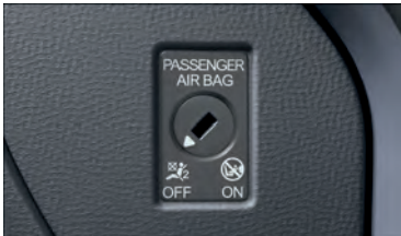
Fig. 35 In the dash panel on the front passenger side: key-operated switch for deactivating and activating the front airbag on the front passenger side
