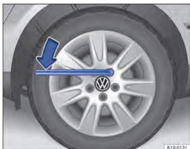
Fig. 191 Changing a wheel: loosening the wheel bolts.
