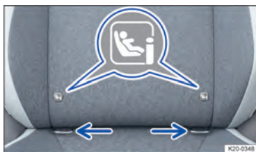
Fig. 45 Markings identifying the i-Size anchorage points for child seats on the front passenger seat.
