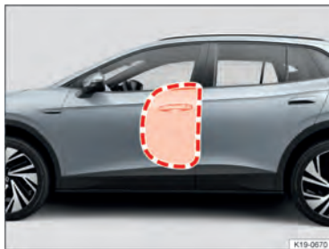
Fig. 36 In the interior on the left-hand side of the vehicle: side airbag deployment zone.
