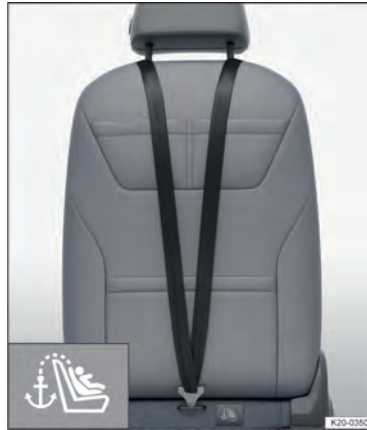
Fig. 48 On the rear of the front passenger seat: attached top tether.
