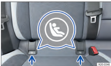
Fig. 43 Markings identifying the ISOFIX anchorage points for child seats on the seats of the rear bench seat.
