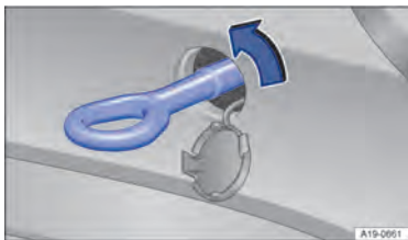
Fig. 172 In the rear bumper on the right: screwing in the towing eye: screwing in the towing eye.
