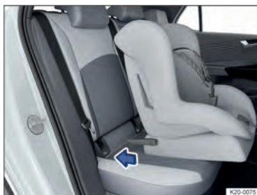
Fig. 46 Illustration: fitting a child seat with the attachment arms.
