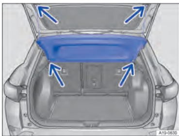
Fig. 125 In the luggage compartment: removing and installing the luggage compartment cover.
