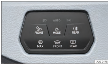
Fig. 86 Next to the steering wheel: touch panel for switching on the exterior lighting.
