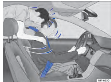
Fig. 24 The unbelted rear passenger is thrown forwards, hitting the belted driver.
