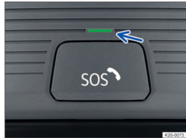
Fig. 51 In the roof console: control for legally required eCall Emergency System (behind button cover).
