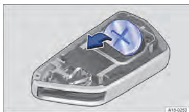
Fig. 56 Vehicle key: replacing the button cell.
