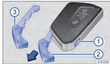
Fig. 54 Vehicle key: releasing the spare key.
