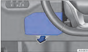
Fig. 162 Left-hand drive vehicle: fuse box cover in the dash panel on the driver side
