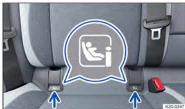
Fig. 44 Markings identifying the i-Size anchorage points for child seats on the seats of the rear bench seat.
