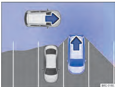
Fig. 119 Illustration of Rear Traffic Alert: monitored area around the vehicle leaving the parking space.
