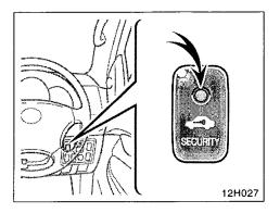
The system is automatically set when the key is removed from the engine switch. The indicator light will start flashing to show the system is set.
