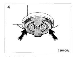
Install the rubber cover as shown, and fit it securely on the boss. Plug in the connector.
