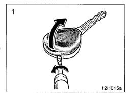
Open the cover using a flathead screwdriver wrapped with plastic tape.
