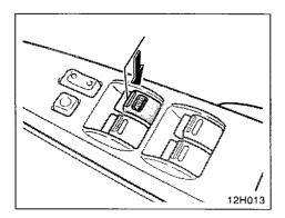
Automatic opening operation: Push the switch completely down and then release it. The window will fully open. To stop the window partway, lightly pull the switch up and then release it.
