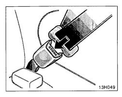
5. To remove the child (convertible) seat, press the buckle release button and allow the belt to retract completely. The belt will move freely again and be ready to work for an adult or older child passenger. Unhook the child restraint attaching clip from the child restraint anchor fitting.
