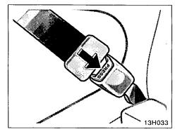
3. To remove the child (convertible) seat, press the buckle release button.
