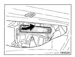
2. Remove the filter cover as shown in the illustration.
