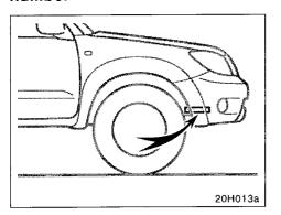
The vehicle identification number (VIN) is the legal identifier for your vehicle. This number is stamped on the front right frame as shown in the illustration.
