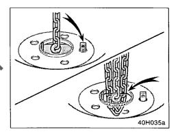
When storing the spare tire, put it in place with the outer side of the wheel facing up and hook the holding bracket as shown in the illustration. After the tire goes half way up, check that the suspended chain is able to enter the tire hole, for proper storage. Then secure the tire, taking care that the tire goes straight up without catching on the chain of any other part, to prevent it from flying during a collision or sudden braking.
