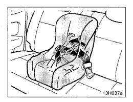
While pressing the child (convertible) seat firmly against the seat cushion and seatback, tighten the lap belt by pulling its free end to hold the child (convertible) seat securely.
