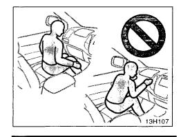
• Do not sit on the edge of the seat or lean against the dashboard when the vehicle is in use, since the front passenger airbag could inflate with considerable speed and force. Anyone who is up against, or very close to, an airbag when it inflates, can be killed or seriously injured. Sit up straight and well back in the seat, and always use your seat belt properly.
