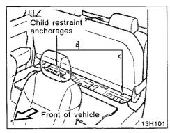
For easy installation of child restraints, your vehicle has two child restraint anchorages under the rear seat cushion.
