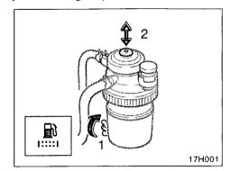
When the fuel system warning light flashes, the water in the fuel filter must be drained immediately.
