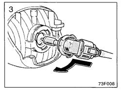
Install the bulb base by turning it clockwise to the front of the vehicle.
