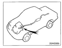
The catalytic converter is an emission control device installed in the exhaust system.
