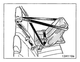
4. Attach the child restraint attaching clip to the child restraint anchor fitting. Make sure the clip is securely attached and tighten the upper anchorage strap. See "—Child restraint anchorages" on page 61 for instructions.
