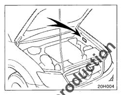
The vehicle identification number (VIN) is also on the manufacturer's plate (shown in the illustration).
