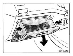
Open the glove box and push in each side of the glove box to release the stoppers.
