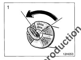
To unlock the fuel tank cap, insert ignition key and turn it counterclockwise.
