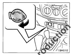
The power outlet is designed for power supply for car accessories. To use it, open as shown.
