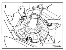
For easy access to the right-hand front turn signal light (except for the 1GR-FE engine): Release the clips of the air cleaner filter cover, and remove both the cover and filter.
