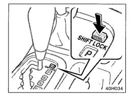
If you cannot move the selector lever out of the "P" position to other positions even though the brake pedal is depressed, use the "SHIFT LOCK" button as follows:
