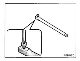
When connecting a jack handle extension with jack handle end, use a Phillips-head screwdriver or your hand to tighten the bolts on the joints as shown in the illustration.
