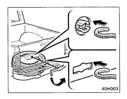
Insert the jack handle end with the extensions into the lowering screw through the access hole and turn it counterclockwise by pushing it to the front lightly.
