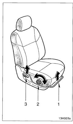
1. SEAT POSITION ADJUSTING LEVER Hold the center of the lever and pull it up. Then slide the seat to the desired
