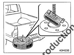
After the tire is lowered completely to the ground, remove the holding bracket as shown in the illustration.
