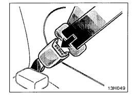
To remove the junior (booster) seat, press the buckle release button and allow the belt to retract.
