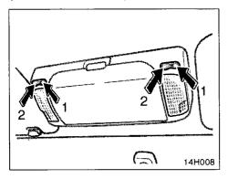
To turn on the personal light, push the switch on side 1. To turn the light off, push the switch on side 2.
