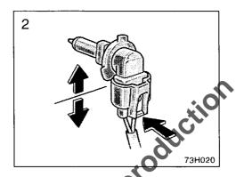
2. Pull the bulb out of the bulb base. If the connector is right, wiggle it.
