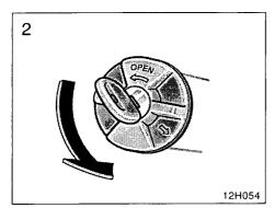
To remove the fuel tank cap, turn the cap slowly counterclockwise, then pause slightly before removing it.
