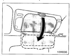
To use the auxiliary box, open as shown in the illustration.
