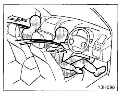
The driver and front passenger seat belt pretensioners (vehicles with separate front seats) or driver and front outside passenger seat belt pretensioners (vehicles with bench front seat) are designed to be activated in response to a severe frontal impact.
