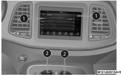
Uconnect 4 With 7-inch Display Buttons On The Touchscreen And Buttons On The Faceplate
