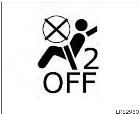
Front passenger air bag and status light
