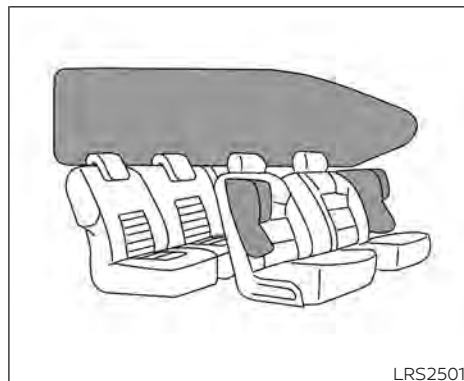
Front seat-mounted side-impact supplemental air bag and roof-mounted curtain side-impact and rollover supplemental air bag systems
