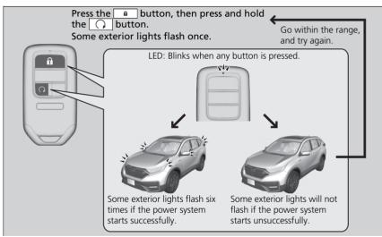
The power system is on for up to 10 minutes without you starting the vehicle. To extend the time for another 10 minutes during the first 10 minutes, press the  $\boxed{10}$  button, then press and hold the  $\boxed{10}$  button.
