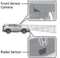
The radar sensor is inside the front arille.
