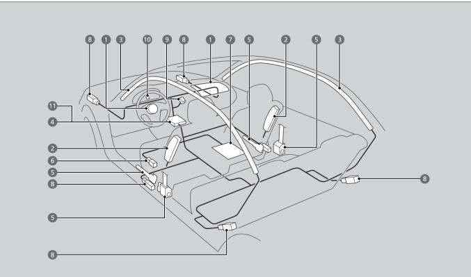
The front, front side, and side curtain airbags are deployed according to the direction and severity of impact. Both side curtain airbags are deployed in a rollover. The airbag system includes:
