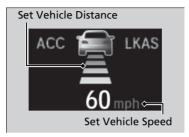
When ACC with Low Speed Follow starts operating, the vehicle icon, distance bars and set speed appear on the driver information interface.
