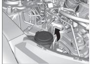
Pour the washer fluid carefully. Do not overflow the reservoir.
