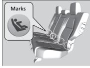
Locate the lower anchors under the marks.
