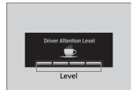
When the (display/information) button is pressed, bars in the Driver Information Interface light up in white to indicate the degree of the driver's attention.
