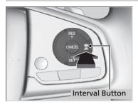
Press the 🖹 (Interval) button to change the ACC with Low Speed Follow followinginterval. Each time you press the button, the followinginterval (the interval behind a vehicle detected ahead of you) setting cycles through extra
