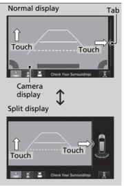
You can switch the display to normal display or split display by touching the tab vicinity or on the camera display.
