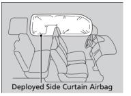
The side curtain airbag is designed to deploy in a rollover or a moderate-to-severe side impact.
