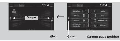
Selecting  $\langle\!\!\langle\!\!\langle n \rangle\!\!\rangle$ , or swiping the screen left or right changes to the next screen.
