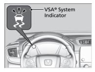
When VSA<sup>®</sup> activates, you may notice that the engine and motor do not respond to the accelerator. You may also notice some noise from the hydraulic system. You will also see the indicator blink.
