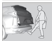
Use a forward and back kicking motion under the center of the rear bumper to open or close the power tailgate while carrying the smart entry remote.
