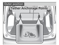
A tether anchorage point is provided behind the rear outer seating position and in the ceiling for the rear center. If you have a child seat that comes with a tether but can be installed with a seat belt, the tether may be used for additional security.
