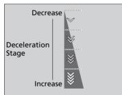
The default deceleration stage is  $\bowtie$ . Each paddle selector operation makes a single stage deceleration change.
