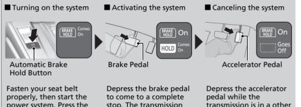
power system. Press the automatic brake hold button.
