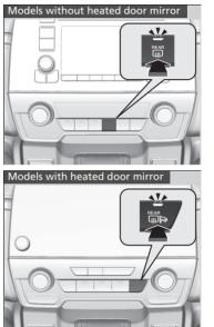
The rear defogger and heated door mirror<sup>\*</sup> automatically switch off after 10-30 minutes depending on the outside temperature. However, if the outside temperature is 32°F (0°C) or below, it does not automatically switch off.
