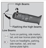
Rotating the light switch turns the lights on and off, regardless of the power mode setting.
