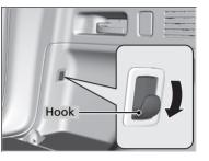
The cargo hook on the driver's side of the cargo area can be used to hang light items.
