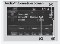
(A): Shows how much time the replayed segment is behind the real-time broadcast(B): Replayed segment
