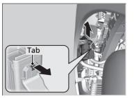
**3.** Pull the tab to remove the fuse box.
