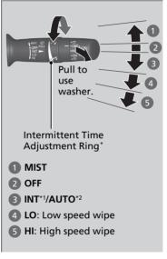
The windshield wipers and washers can be used when the power mode is in ON.
