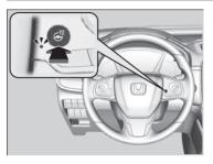
The power mode must be in ON to use the heated steering wheel.
