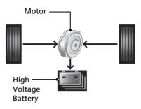
When decelerating without the accelerator being depressed or the brake pedal being applied, or while driving downhill, the electric motor acts as a generator that recovers a portion of the electrical energy that was used to accelerate the vehicle. This regenerative braking slows the vehicle in a manner similar to engine braking in a gasoline-powered vehicle. You can control the rate of deceleration by using the deceleration paddle selector.
