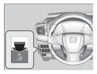
Press and hold the button until the beeper sounds to switch the system on or off.
