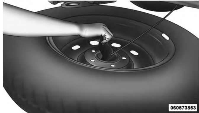
Reinstalling The Retainer
