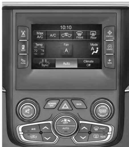
5.0 With Automatic Temperature Controls
