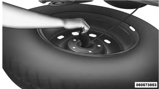
Reinstalling The Retainer
