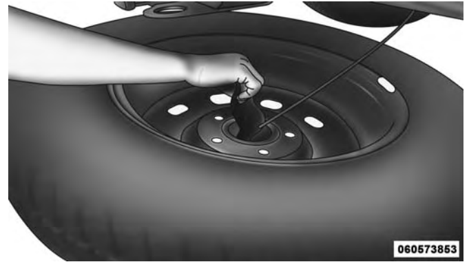
Pulling The Retainer Through The Center Of The Wheel
