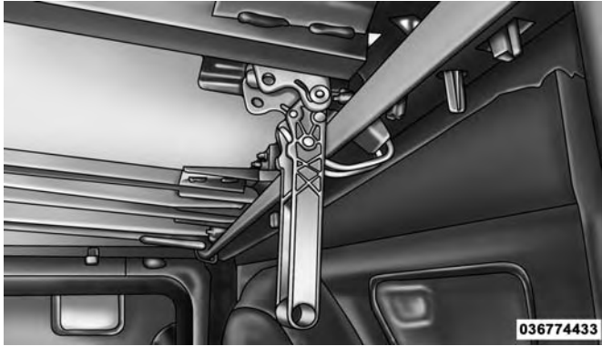
Semi Clamped Position
