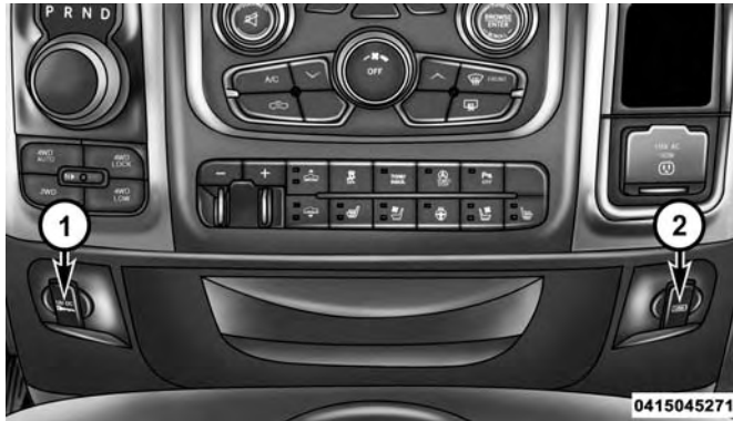
Power Outlets — Center Stack
