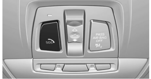
SOS button in the roofliner
