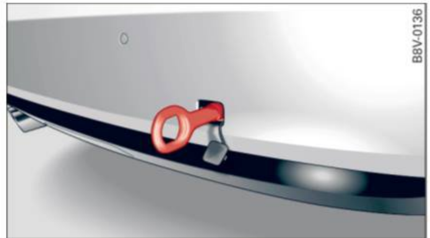
Fig. 193 Right rear towing loop: towing loop installed
