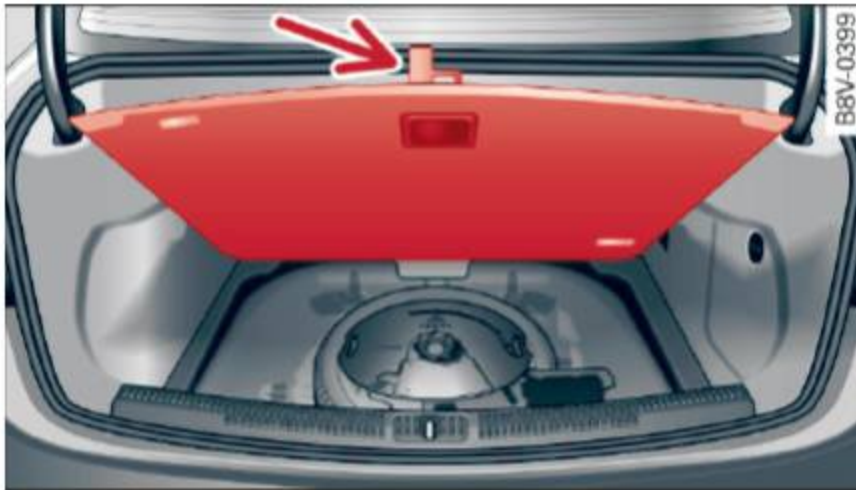
Fig. 174 Luggage compartment: cargo floor cover folded upward
