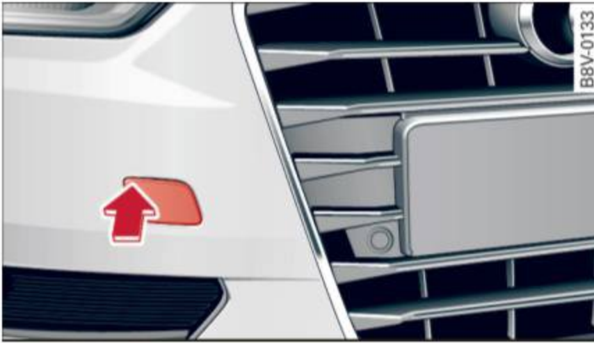
Fig. 190 Right front bumper: removing the cover
