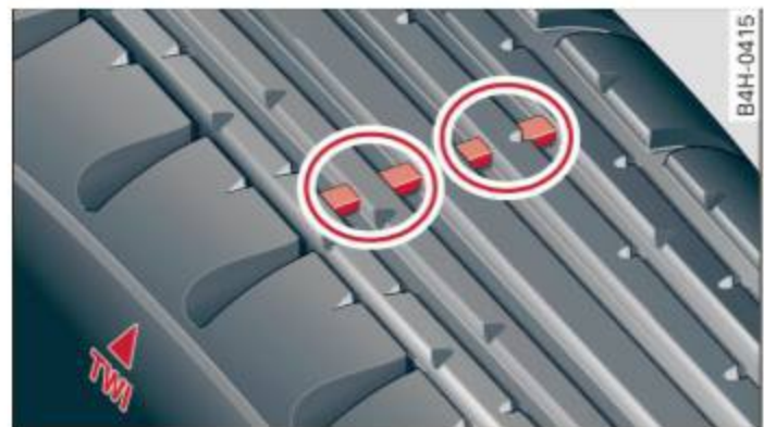
Fig. 169 Tire profile: treadwear indicator
