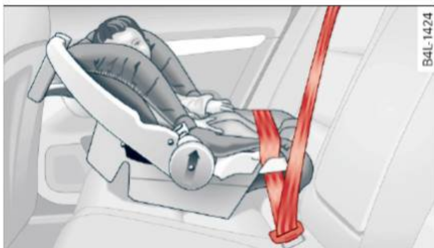
Fig. 139 Schematic overview: rearward-facing infant seat, properly installed on the rear seat
