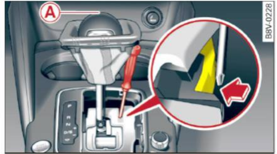
Fig. 78 Selector lever: using the emergency release to move out of the Park position
