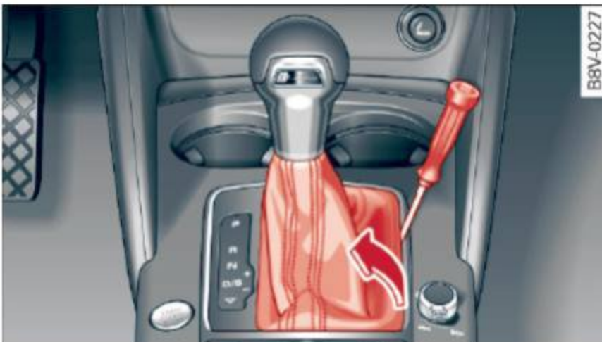
Fig. 77 Selector lever: removing the cover
