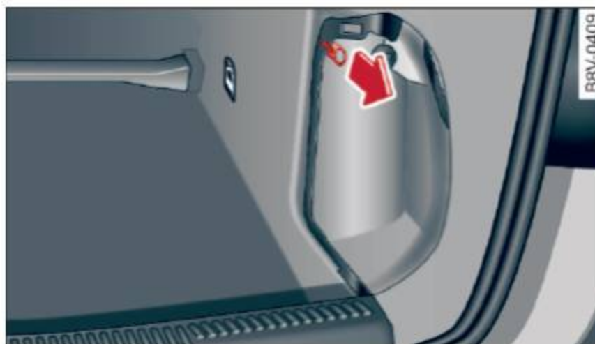
Fig. 151 Right rear luggage compartment: emergency release
