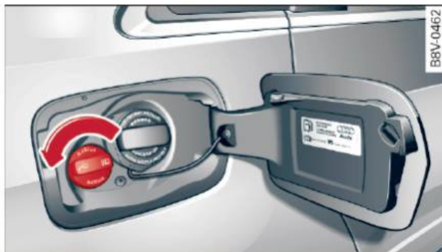
Fig. 153 Right rear vehicle side: removing the AdBlue cap
