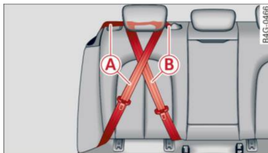
Fig. 138 Schematic overview: keep unused safety belts away from children in child safety seats. A - outer rear safety belt, B - center rear safety belt*
