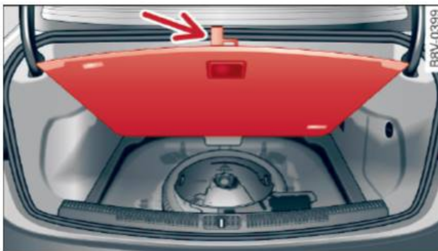
Fig. 182 Luggage compartment: cargo floor cover folded upward
