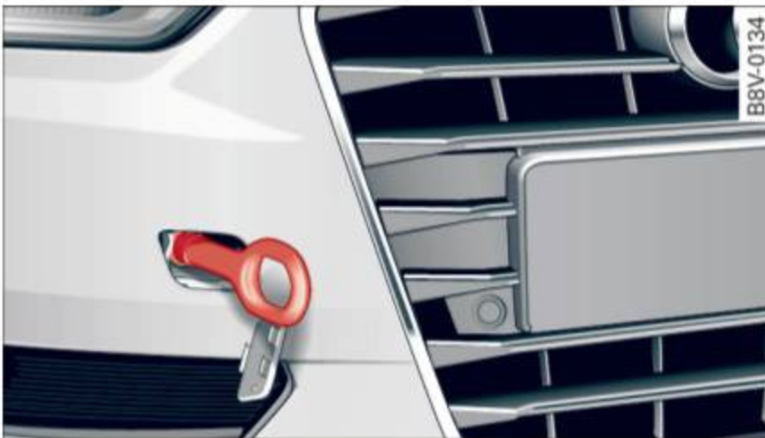
Fig. 191 Right front bumper: towing loop installed
