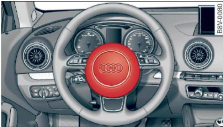
Fig. 128 Location of driver airbag: in steering wheel
