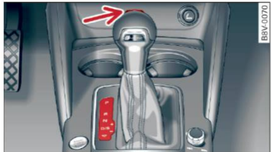
Fig. 74 Section of the center console: selector lever with interlock button
