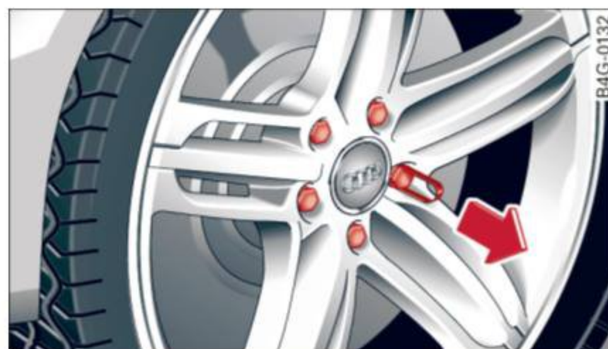
Fig. 176 Changing a wheel: removing the wheel bolt caps
