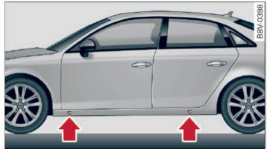
Fig. 178 Sill panels: markings
