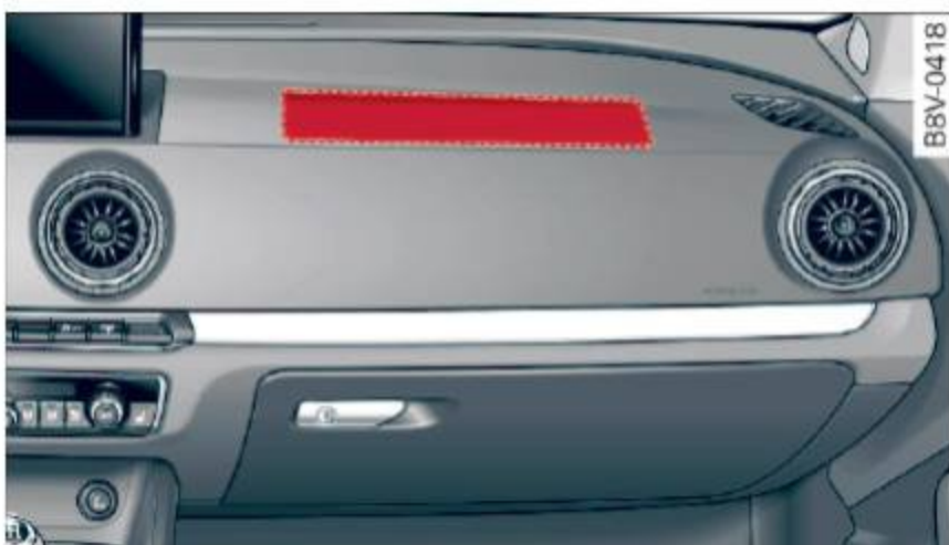
Fig. 129 Location of front passenger's airbag: in the instrument panel
