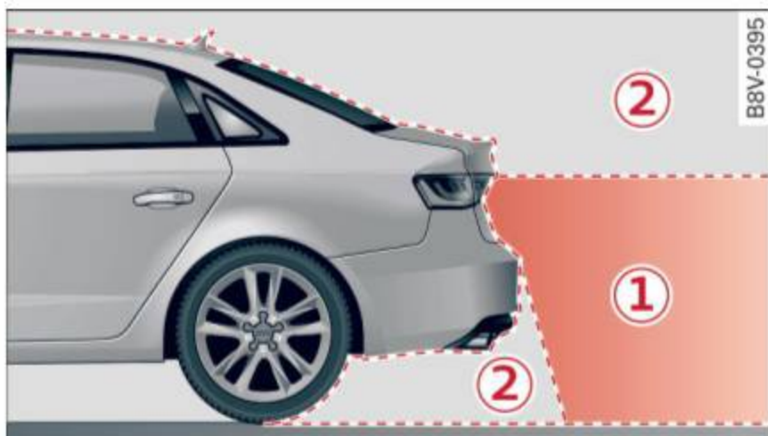
Fig. 106 Area covered ① and area not covered ② by the rearview camera.
