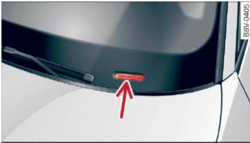
Fig. 197 Vehicle Identification Number (VIN) plate: location on driver's side dash panel
