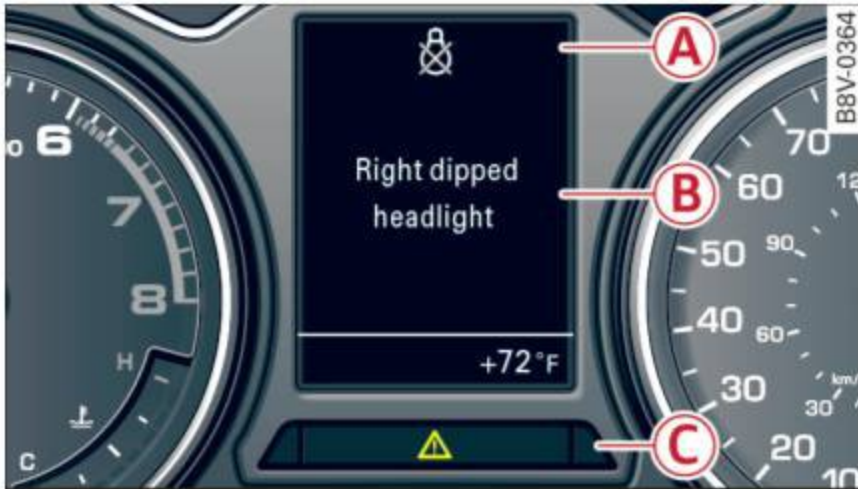
Fig. 6 Instrument cluster: example of a display in vehicles with a monochrome display
