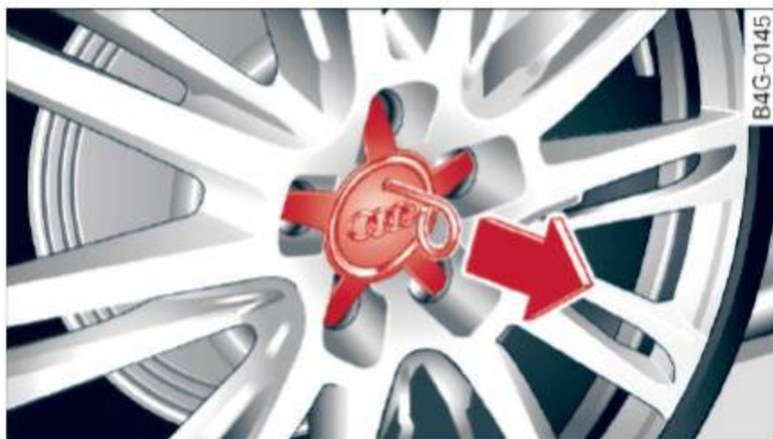
Fig. 175 Changing a wheel: Removing the wheel cover
