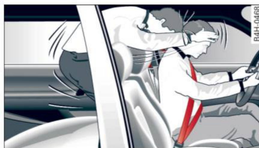
Fig. 120 A rear passenger not wearing a safety belt will fly forward and strike the driver
