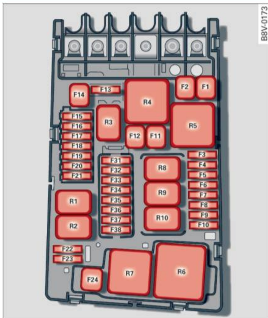
Fig. 187 Engine compartment: fuse assignment
