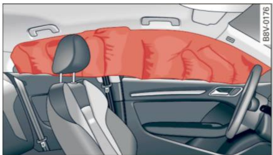
Fig. 137 Illustration of principle: Inflated side curtain airbags on the left side
