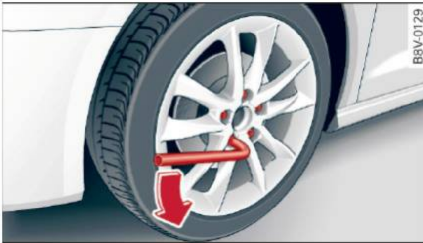
Fig. 177 Changing a wheel: loosening the wheel bolts
