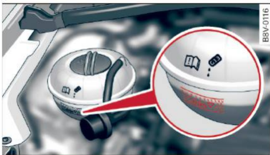
Fig. 162 Engine compartment: markings on the coolant expansion tank
