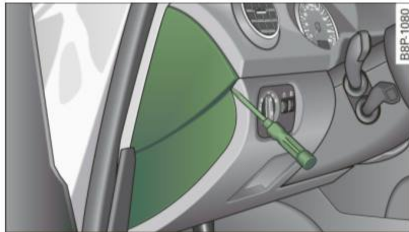
Fig. 213 End face of instrument panel: removing cover plate to access fuses
