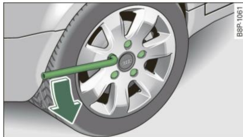
Fig. 206 Wheel change: loosening the wheel bolts
