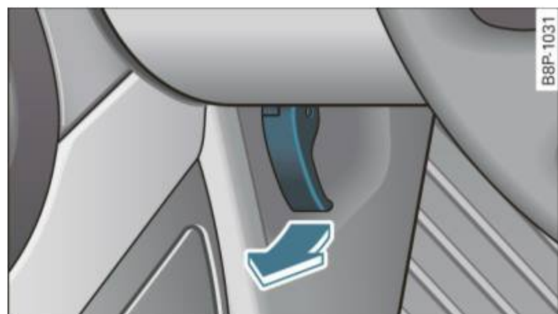
Fig. 182 Driver's side footwell: engine hood release lever
