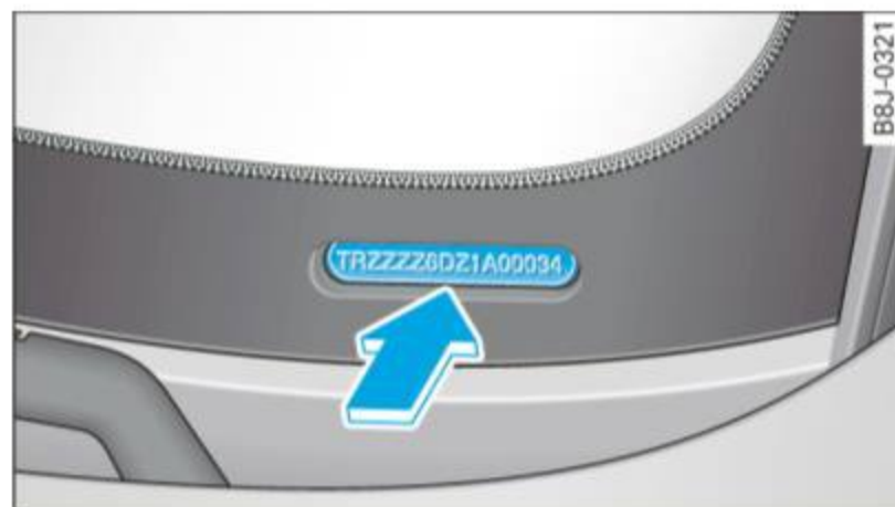
Fig. 227 Vehicle Identification Number (VIN) plate: location on driver's side dash panel
