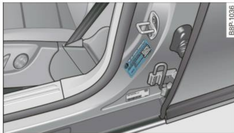
Fig. 195 Tire pressure label: located either on driver's side B-pillar or inside the fuel filler flap
