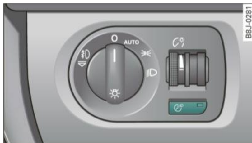
Fig. 72 Dashboard detail: coming home/leaving home switch beside light switch
