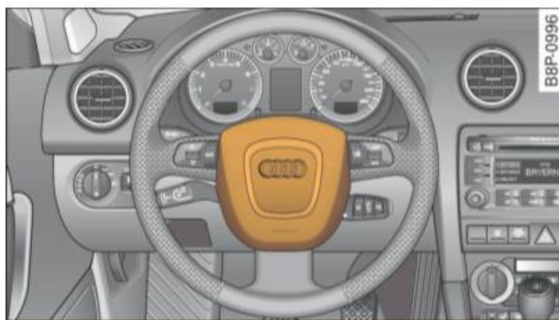
Fig. 158 Location of driver airbag: in steering wheel
