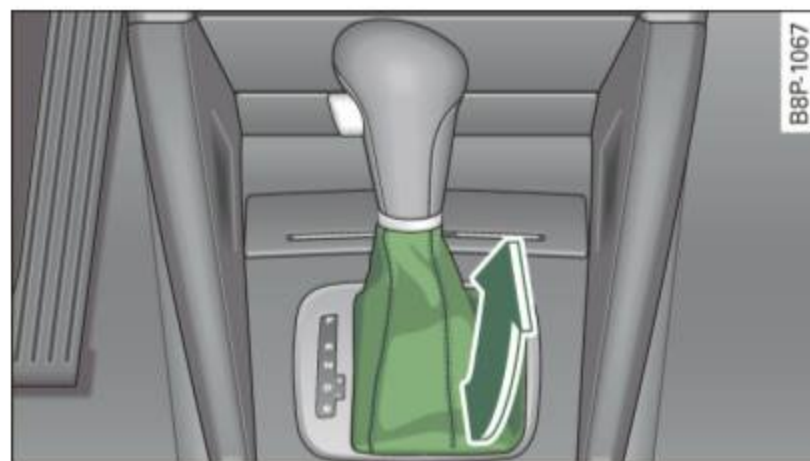
Fig. 211 Selector lever: removing the selector lever boot
