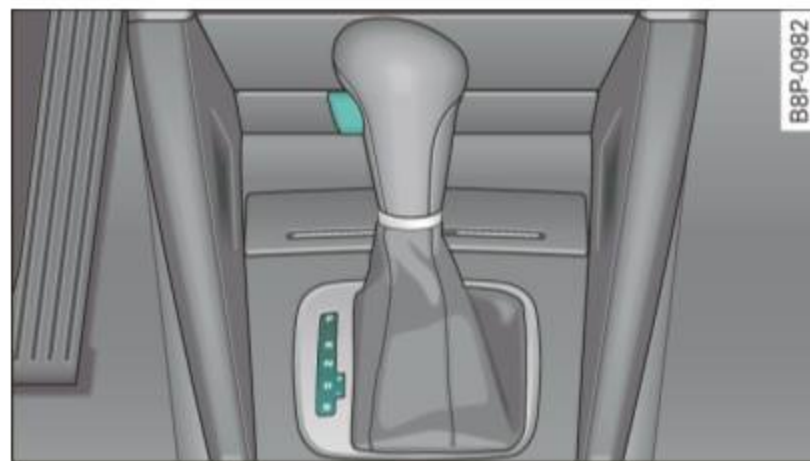
Fig. 137 Section from center console: Selector lever with release button
