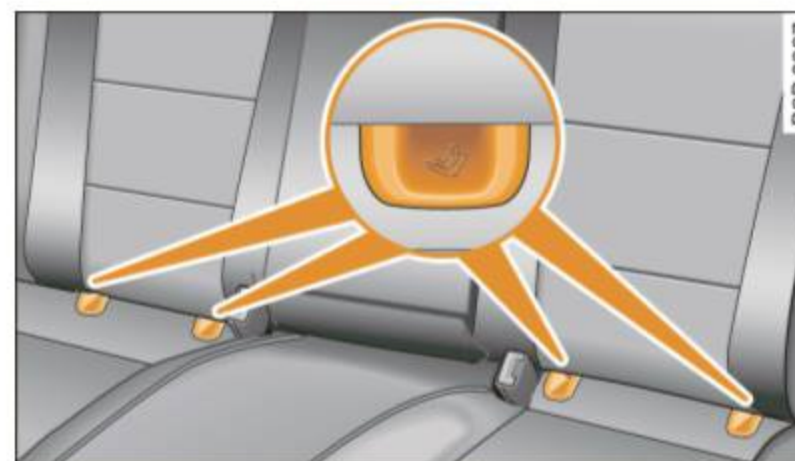
Fig. 173 Installation of child safety seat with rigid latches on bars
