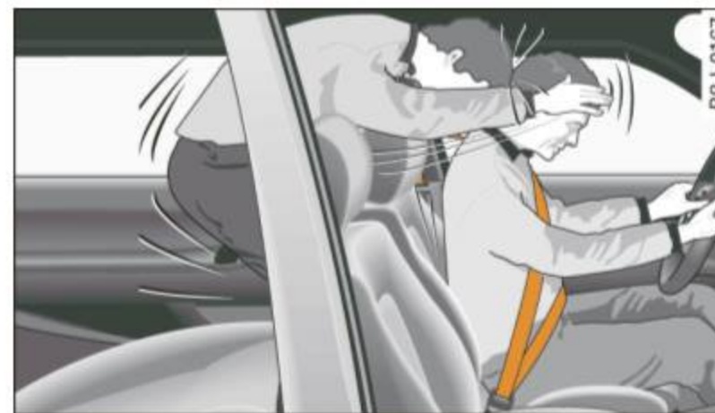
Fig. 151 A rear passenger not wearing a safety belt will fly forward and strike the driver
