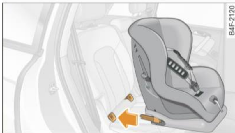
Fig. 172 LATCH-type seat with both latch bars extended
