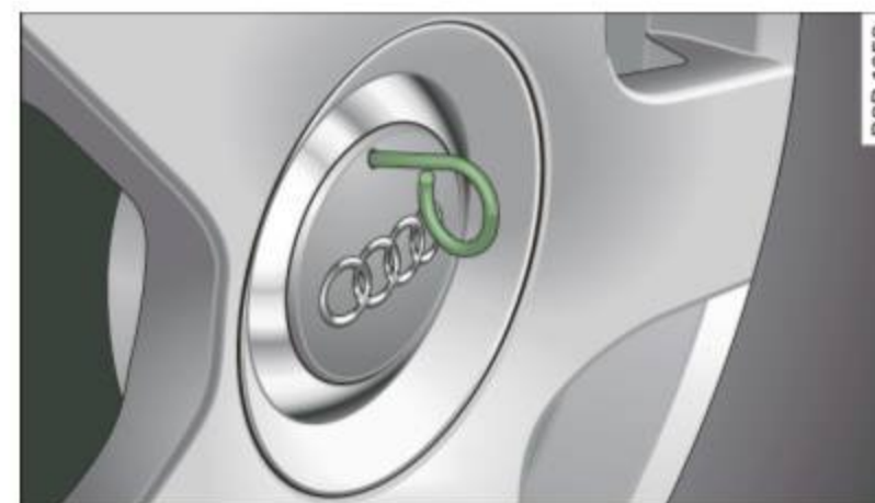
Fig. 203 Wheel change: removing the wheel cover
