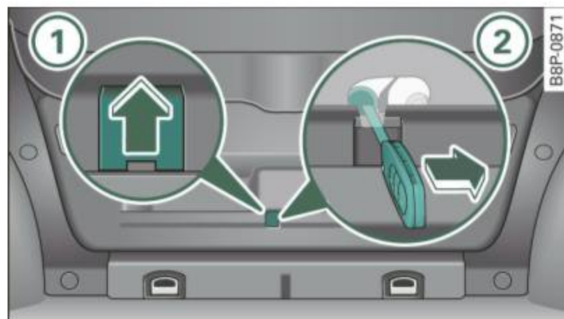
Fig. 53 Rear lid interior section: Emergency release
