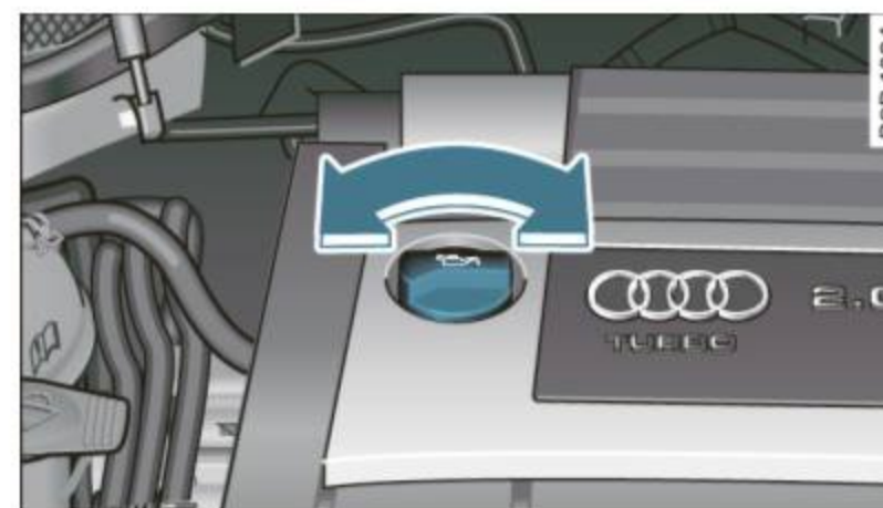
Fig. 188 Oil filler cap location: 2.0 liter, 4- cylinder turbo engine
