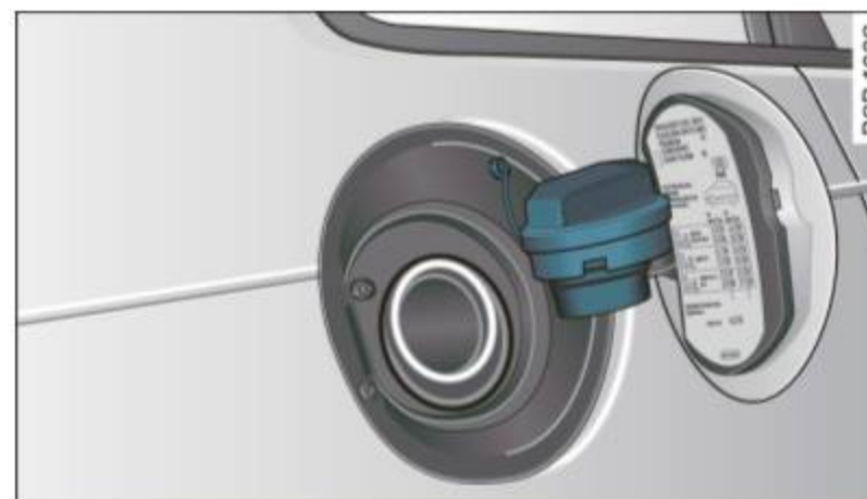
Fig. 180 Fuel cap hooked on the opened fuel filler flap
