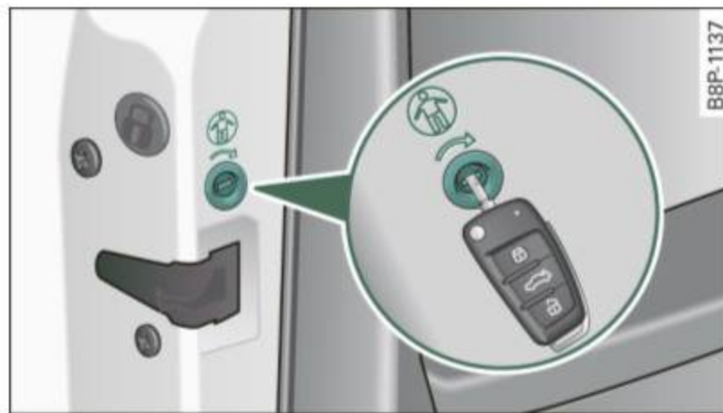
Fig. 55 Rear doors: child safety lock
