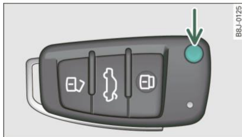
Fig. 43 Fold-up master key with remote control
