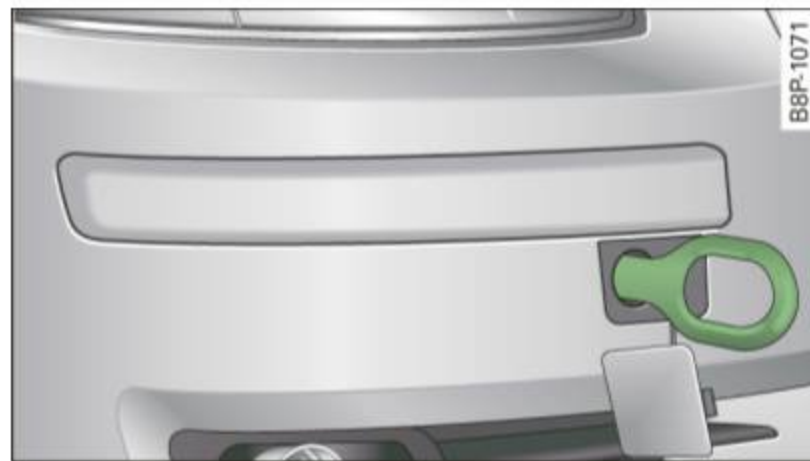
Fig. 221 Front bumper: screwing in the towing loop
