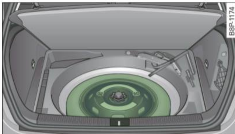
Fig. 202 Compact spare wheel in the wheel well
