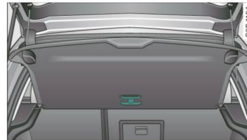
Fig. 107 Mounting hooks under the rear parcel shelf
