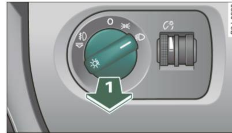
Fig. 71 Fog light activation: light switch position on vehicles WITHOUT sensor light
