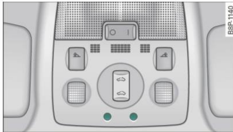
Fig. 78 Control panel above windshield: position of ambient light bulbs
