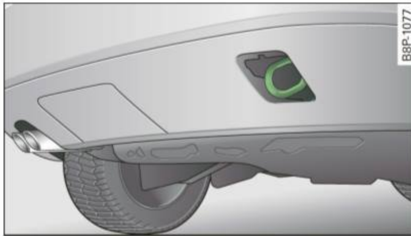
Fig. 223 Rear bumper: towing loop inserted
