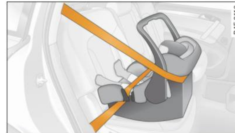
Fig. 166 Rearward-facing infant seat, properly installed on the rear seat
