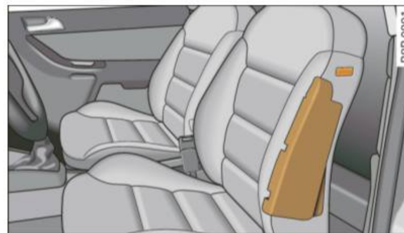
Fig. 162 Side airbag location in the driver's seat
