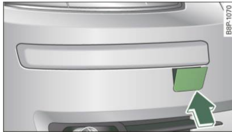
Fig. 220 Front bumper: removing the cover cap
