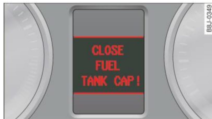
Fig. 16 Center display: fuel filler cap open
