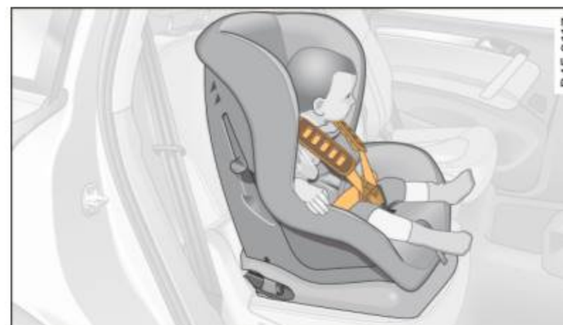
Fig. 167 Rear seat: smaller child in a properly installed forward-facing convertible child safety seat
