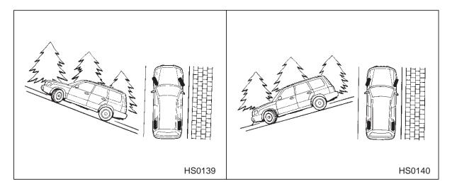
When parking on a hill, always turn the steering wheel. When the vehicle is headed up the hill, the front wheels should be turned away from the curb. When facing downhill, the front wheels should be turned into the curb.
