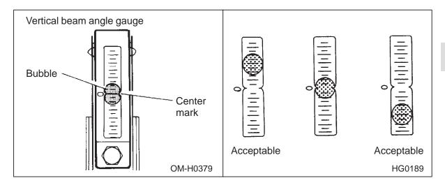
1. Look at the vertical beam angle gauge. The bubble on the gauge should not deviate from the center of the gauge by more than four segments on either side of the gauge.
