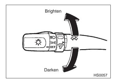
When the lighting switch is in the "  $\stackrel{*}{>}$ 0  $\stackrel{*}{=}$  or "  $\stackrel{*}{=}$ 0" position, you can adjust brightness of the instrument panel illumination for better visibility. To brighten, turn the control dial counterclockwise. To darken, turn the control dial clockwise.
