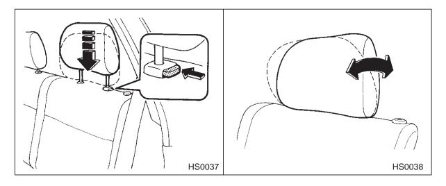
To raise the head rest, pull it up. To lower it, push the head rest down while depressing the release button on the top of the seatback.
