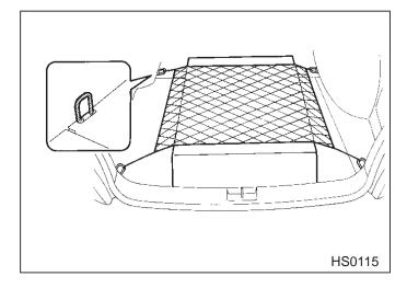
The luggage compartment is equipped with four anchorage eyelets so that luggage can be secured with a luggage net or ropes.
