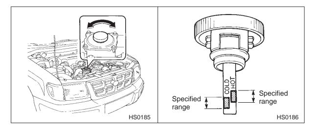
4. Remove the dipstick again and check the fluid level on it. If it is below the lower level of the "HOT" range, add the recommended steering fluid up to the specified range of the dipstick.
