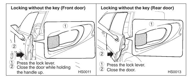
To lock the **front door** from the outside without the key, press the end of the lock lever down on the door and hold the outside door handle up while closing the door.
