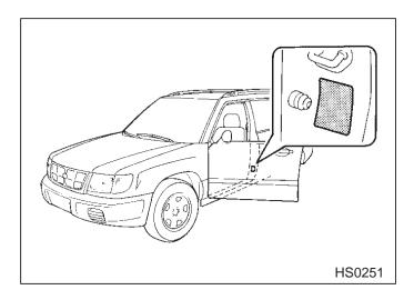
The recommended tire pressure and sizes are provided on the tire placard, which is located under the door latch on the driver's side.
