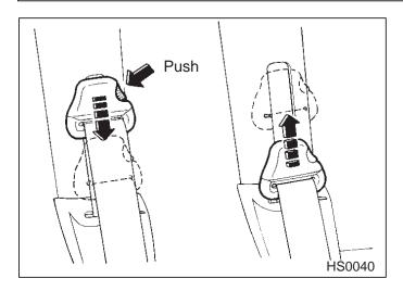
The shoulder belt anchor height should be adjusted to the position best for you. To lower the anchor height, push the release button and slide down. To raise the anchor height, slide it up. Pull down on the anchor to make sure that it is locked in place.
