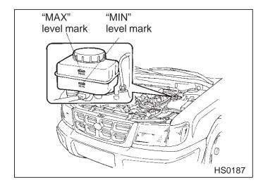
Check the fluid level on the outside of the reservoir. If the level is below "MIN", add the recommended brake fluid to "MAX". Use only brake fluid from a sealed container.
