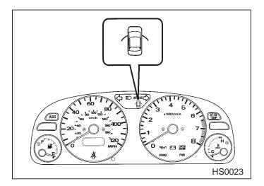
The door open warning light comes on if any door is not fully closed. Always make sure this light is out before starting to drive.
