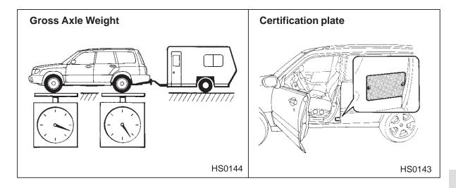
To check both GVWR and GAWR and to confirm that the total weight and weight distribution are within safe driving limits, you should have your vehicle and trailer weighed at a commercial weighing station. Be sure that all cargo is firmly secured to prevent a change in weight distribution while driving.
