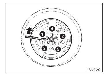
The torque for tightening the nuts is 58 to 72 ft-lb (78 to 98 N-m, 8 to 10 kg-m). This torque is equivalent to applying about 88 to 110 lbs (40 to 50 kg) at the top of the wheel nut wrench. Never use your foot on the wheel nut wrench or a pipe extension on the wrench because you may exceed the specified torque. Have the wheel nut torque checked at a nearest automotive service facility.
