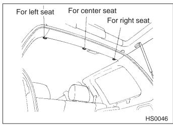
Anchor installation points are located under the covers at the rear edge of the roof.
