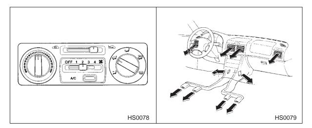
This setting allows you to direct air of different temperatures from the instrument panel and outlets. The air from the foot outlets is slightly
