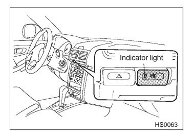
To turn on the outside mirror defogger, push the switch. To turn it off, push the switch again.
