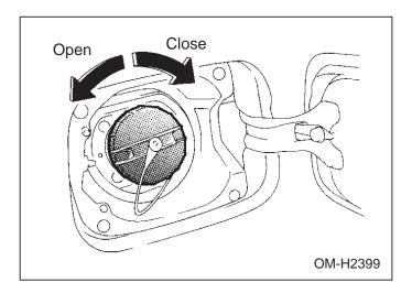
To take off the fuel filler cap, turn it slowly counterclockwise and remove the cap.
