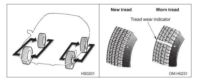
A tire should be replaced when the tread wear indicator appears as a solid band across the tread. The indicators appear when the remaining tread has been worn to 0.063 in (1.6 mm) or less.
