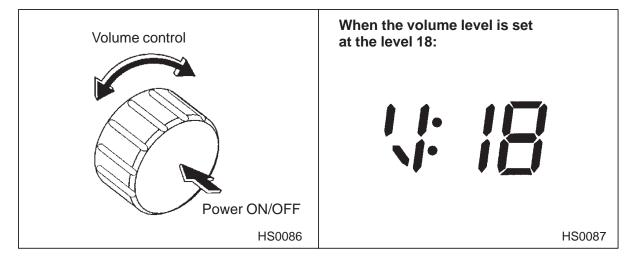
The same knob is used for both power (on/off) and volume control. The radio is turned on and off by pushing the knob and the volume is controlled by turning the knob.
