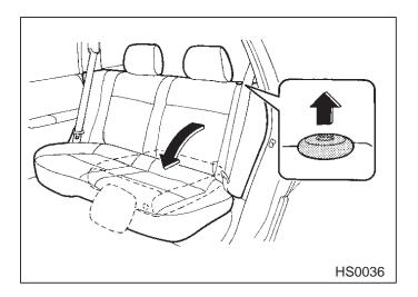
Unlock the seatback by pulling the release knob and fold it down. Then push the seatback downward until it locks into place and make sure that it is securely locked.
