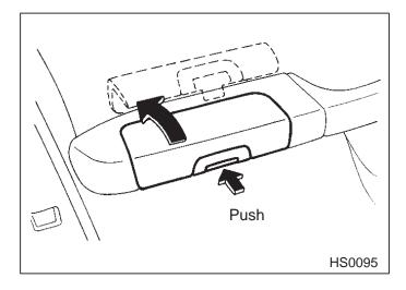
Each door is equipped with a door storage compartment. To open the compartment, push the button and pull up on the lid.
