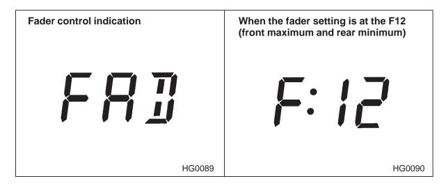
Select the Fader control mode by pressing the "T/B" button. In the fader control mode, the display shows the indication as shown.
