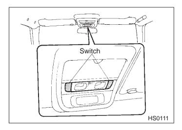
To turn on the spotlight, push the switch. To turn it off, push the switch again.
