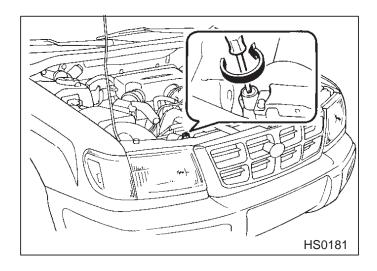
5. Remove the air vent plug from the radiator.
