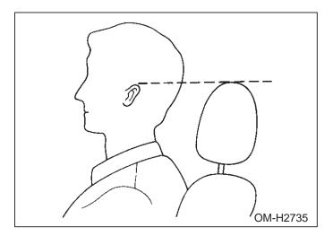
The best position for the head restraint is just above or level with the top of the ears.
