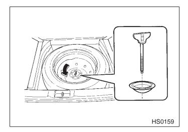
The spare tire is stored under the floor of the luggage compartment. To remove the spare tire, first open the spare tire cover and remove the storage tray, turn the attaching bolt counterclockwise, then take the spare tire out.
