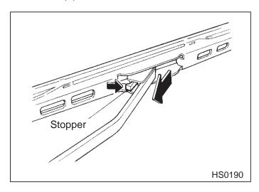
3. Grasp the locked end of the blade rubber assembly and pull it firmly until the stoppers on the rubber are free of the metal support.
