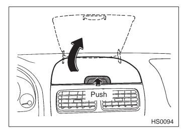
To open the dashboard compartment, push the button and pull up on the lid. Be sure to close the compartment fully before driving.
