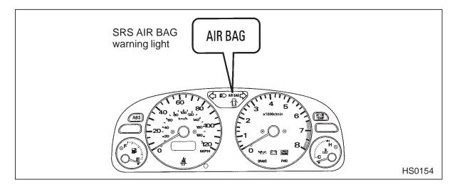
A diagnostic system continually monitors the readiness of the SRS AIR-BAG while the vehicle is being driven. The SRS AIRBAG warning light will show normal system operation by lighting for about 6 seconds when the ignition key is first turned to the "ON" position and then turning off.
