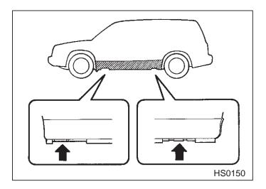
8. Insert the jack handle into the jackscrew, and turn the handle clockwise until the tire clears the ground. Do not raise the vehicle higher than necessary.
