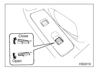
To open the window, push the switch down and hold it until the window reaches the desired position. To close the window, pull the switch up and hold it until the window reaches the desired position.
