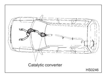
The catalytic converter is installed in the exhaust system. It serves as a catalyst to reduce HC, CO and NOx in exhaust gases, thus providing cleaner exhaust.
