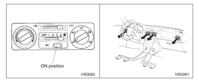
For cooling and dehumidification of the passenger compartment, air flows through the instrument panel outlets:
