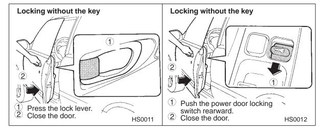
To lock the door from the outside without the key, press the end of the lock lever down on the door and then close the door.
