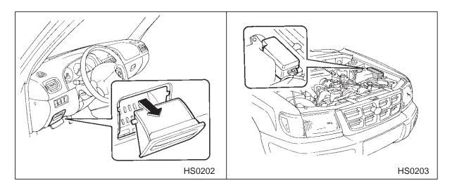
The fuses are designed to melt during an overload to prevent damage to the wiring harness and electrical equipment. The fuses are located in two fuse boxes.
