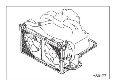
Your vehicle employs an electric cooling fan which is thermostatically controlled to operate when the engine coolant reaches a specific temperature.
