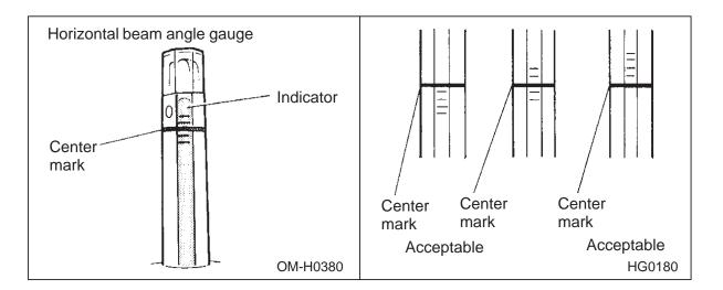
2. Look at the horizontal beam angle gauge. The center mark (the red line on the inner scale) should not deviate from red line on the outer case by more than two segments on either side of the gauge.
