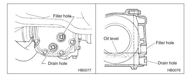
Remove the plug from the filler hole and check the oil level. The oil level should be kept even with the bottom of the filler hole. If the oil level is below the bottom edge of the hole, add oil through the filler hole to raise the level.
