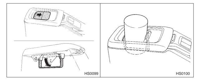
The front passenger's cup holder is built in the lid of the center console. To use the cup holder, open the lid by sliding it forward and unfold the arm. Adjust the opening area by sliding the lid forward or rearward to fit the cup. When not in use, fold the arm and close the lid.
