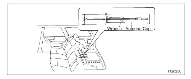
The antenna and the special wrench for mounting/dismounting the antenna is stored in the luggage floor storage tray at the front side.
