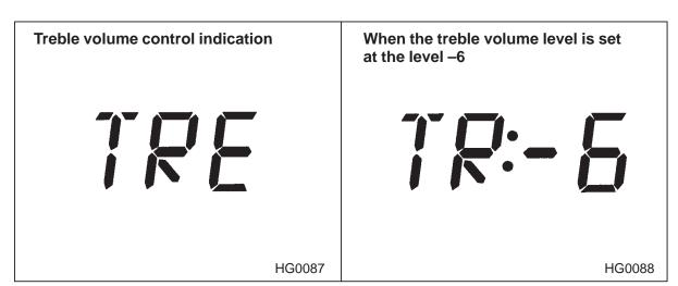
Select the Treble control mode by pressing the "T/B" button. In the treble control mode, the display shows the indication as shown.
