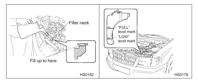
6. Slowly pour the coolant and fill to the radiator filler neck and to the reserve tank's "FULL" level mark. Do not pour the coolant too quickly, as this may lead to insufficient air bleeding and trapped air in the system.
