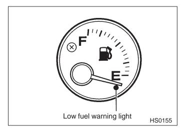
The fuel gauge shows approximately the amount of the fuel remaining in the tank.
