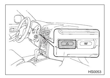
The hazard warning flasher is used to warn other drivers when you have to park your vehicle under emergency conditions. The hazard warning flasher works with the ignition switch in any position.
