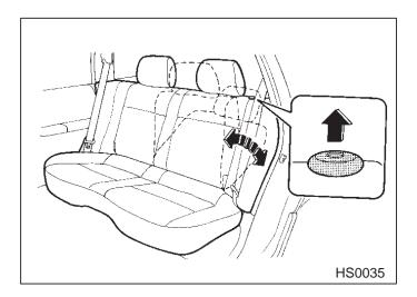
Pull the release knob up and adjust the seatback to the desired position. Then release the knob and make sure the seatback is securely locked into place.
