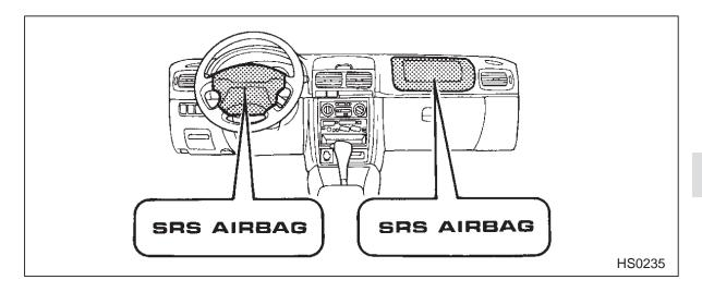
The driver's side SRS AIRBAG is stored in the center portion of the steering wheel. The passenger's side SRS AIRBAG is stored near the top of the dashboard under the cover marked "SRS AIRBAG".
