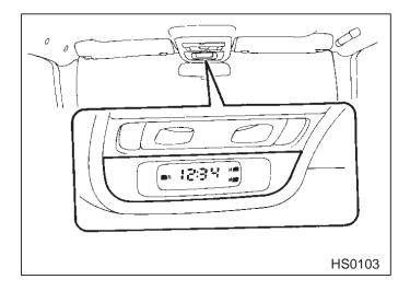
The clock displays the time when the ignition switch is in the "ACC" or "ON" positions.
