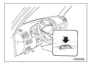
The parking light switch operates regardless of the ignition switch position.
