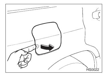
To open the fuel filler door, pull it outward. After refueling, be sure to close the fuel filler door completely.
