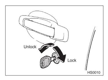
To lock the door from the outside with the key, turn the key toward the rear. To unlock the door, turn the key toward the front.
