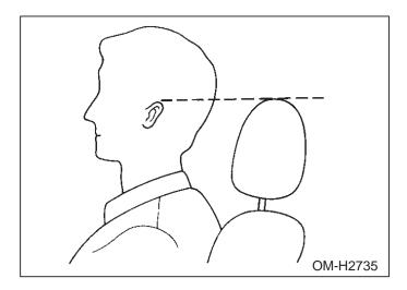
The best position for the head rest is just above or level with the top of the ears.
