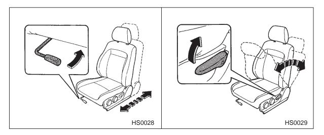
Pull the lever upward and slide the seat to the desired position. Then release the lever and move the seat back and forth to make sure that it is securely locked into place.
