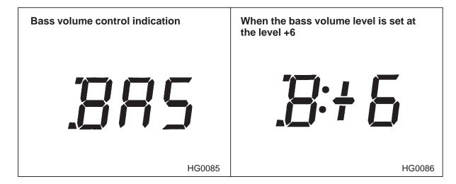
Select the Bass control mode by pressing the "T/B" button. In the bass control mode, the display shows the indication as shown.
