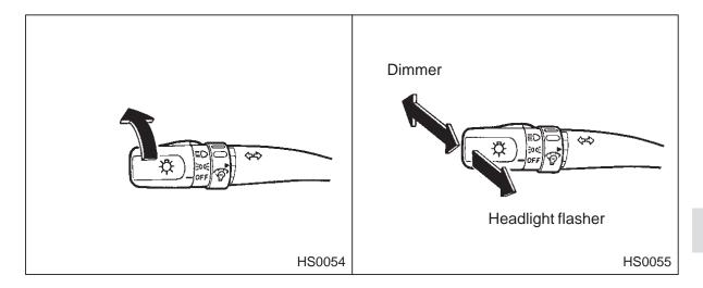
The light switch operates only when the ignition switch is in the "ON" position.
