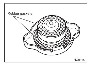
3. After refilling the reserve tank and the radiator, reinstall the caps and check that the rubber gasket inside the radiator cap is in the proper position.
