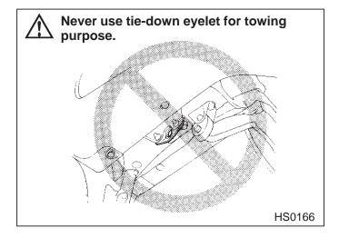
The towing eyelets should be used only in an emergency (e.g., to free a stuck vehicle from mud, sand or snow).
