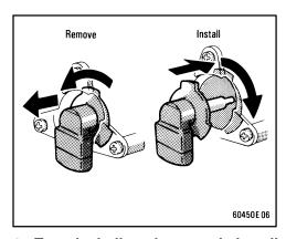
3. Turn the bulb and remove it. Install the new bulb and install the connector.
