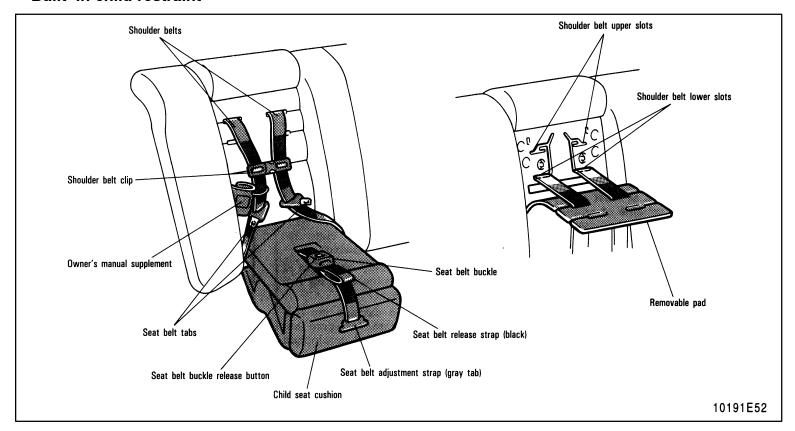
The built-in child restraint system mainly consists of a child seat integrated in the rear seat and 5-point seat belts. Refer to the illustration to become familiar with the parts of the system. This child restraint system conforms to U.S. Motor Vehicle Safety Standard No.213 and Canada Motor Vehicle Safety Standard No.213.4.
