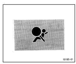
This SRS airbag system has a service reminder indicator to inform the driver of operating problems. If either of the following conditions occurs, this indicates a malfunction of the airbags. Contact your Toyota dealer as soon as possible to service the vehicle.
