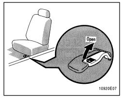
1. To open the fuel filler door, pull the lever up.
