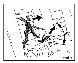
2. While pulling the seat belt release strap (black), pull both shoulder belts together.
