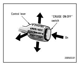
The cruise control allows you to cruise the vehicle at a desired speed over 40 km/h (25 mph) even with your foot off the accelerator pedal.
