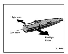
For high beam, push the lever away from you. Pull it toward you for low beam. For the headlight flasher, pull it further back.
