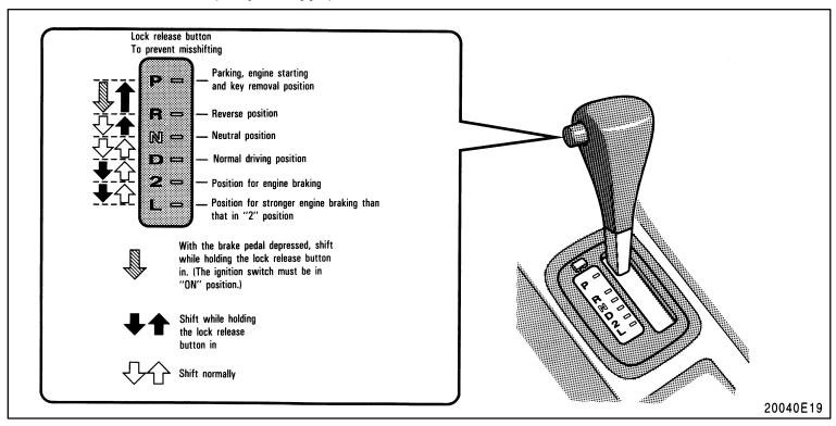
Vehicles with cruise control – When the cruise control is being used, even if you downshift the transmission, engine braking will not be applied because the cruise control is not cancelled. For ways to decrease the vehicle speed, see "Cruise control" in this chapter.
