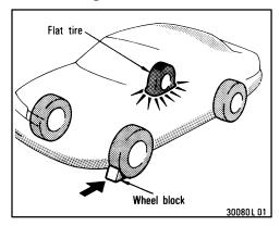
Block the wheel diagonally opposite the flat tire to keep the vehicle from rolling when it is jacked up.
