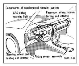
The airbag sensor assembly consists of a safing sensor and airbag sensor.
