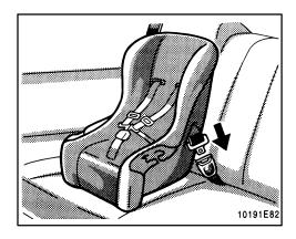
A forward-facing child restraining system should be put on the front seat only when it is unavoidable. Always move the seat as far back as possible, because the force of a deploying airbag could cause death or serious injury to the child.
