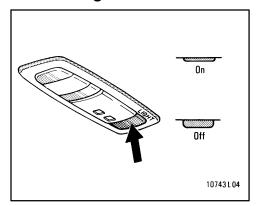
To turn on the personal light, push the switch. To turn it off, push the switch once again.
