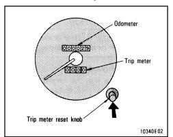
The odometer records the total distance the vehicle has been driven. The trip meter may be set to zero to record the distance on each trip. To reset the trip meter, press the trip meter reset knob.
