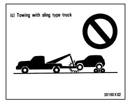
(c) Towing with sling type truck
