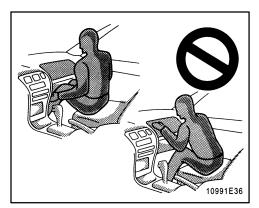
Do not sit on the edge of the seat or lean over the dashboard when the vehicle is in use. The airbags inflate with considerable speed and force; you may be killed or seriously injured. Sit up straight and well back in the seat, and always use your seat belt.
