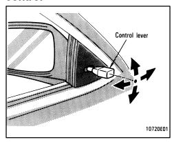
To adjust the rear view mirror, simply operate the control lever.
