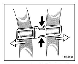
Compress the shoulder belt clip to separate the right and left shoulder belts.
