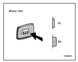
Make sure you turn the defogger off when the window is clear. Leaving the defogger on for a long time could cause the battery to discharge, especially during stop-and-go driving. The defogger is not designed for drying rain water or for melting snow.
