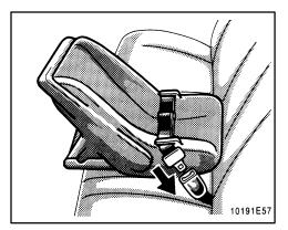
Run the center lap belt through or around the infant seat following the instructions provided by its manufacturer and insert the tab into the buckle taking care not to twist the lap belt.
