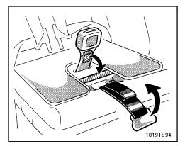
9. To store the built-in child restraint, fasten the shoulder belt clip and return the seat belt buckle using the fastener tapes. Fold up the seat belt adjustment strap (gray tab) in the seat so that the edge of the strap does not come out of the raised seat cushion. Raise the seat cushion and return the head pad by engaging the fastener tapes while pressing the child restraint cushion and head pad firmly.
