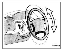
To change the steering wheel angle, pull up the lock release lever, tilt the steering wheel to the desired angle and release the lever.
