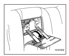
Add slack to the shoulder belts by pulling both of them together while pulling the black seat belt release strap (see step 4 for illustrated instruction). Then pull down the seatback part of the removable pad. Determine the proper shoulder belt slot height for your child. Select the slots at or just above the top of the child's shoulders.
