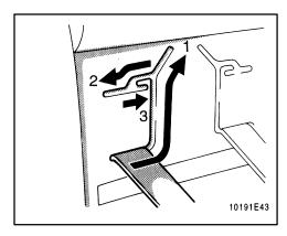
To move the shoulder belts from the lower slot to the upper slot:
