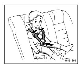
8. To release the child from the seat belts, separate the shoulder belt then press the buckle release button.
