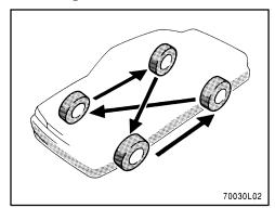
To equalize tire wear and help extend tire life, Toyota recommends that you rotate your tires every 12000 km (7500 miles). However, the most appropriate timing for tire rotation may vary according to your driving habits and road surface conditions
