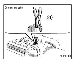
Do not connect it to or near any part that moves when the engine is cranked.
