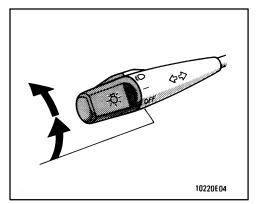
To turn the lights on, twist the knob on the end of the lever.
