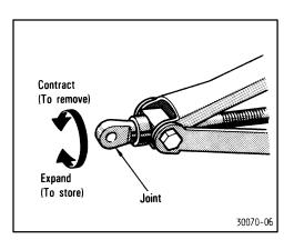
When removing the jack, turn the joint by hand towards the CONTRACT direction until the jack is free. When storing, turn the joint by hand towards the EXPAND direction until the jack is firmly secured to prevent it from flying forward during a collision or sudden braking.
