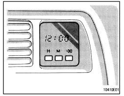
The digital clock indicates the time with the ignition key at the "ACC" or "ON" position. To reset the hour, depress the "H" button. To reset the minutes, depress the "M" button. To adjust the time to full hour, depress the ":00" button.
