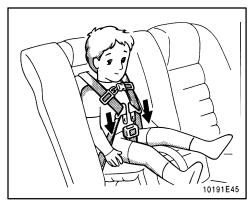
Sit the child on the child seat. Place a shoulder belt over each shoulder. Insert the tabs into the buckle.
