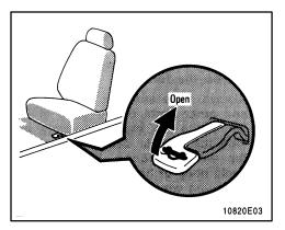
To open the trunk lid from the driver's seat, pull up on the lock release lever.
