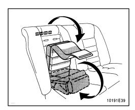
Separate the fastener tapes behind the head restraint to separate the head pad from the seatback. Lower the child restraint cushion and fold back the head pad under the child restraint cushion.
