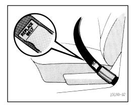
Replace the font seat belt if the warning label under the sleeve can be seen. The warning label, "RE-PLACE BELT", will appear if the belt receives a severe impact or other force.
