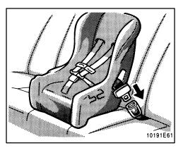
1. Run the center lap belt through or around the convertible seat following the instructions provided by its manufacturer and insert the tab into the buckle taking care not to twist the lap belt.
