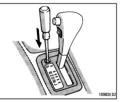
3. Insert the screwdriver or equivalent into the hole to push down the shift lock override button. You can shift out of "P" position only while pushing the button.
