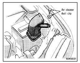
1. Open the hood. LEFT SIDE HEADLIGHT: Remove the clip and take out the air cleaner duct.
