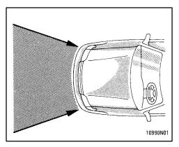
However, this threshold velocity will be considerably higher if the vehicle strikes an object, such as a parked vehicle or sign pole, which can move or deform on impact, or if it is involved in an underride collision (e.g. a collision in which the nose of the vehicle "underrides", or goes under, the bed of a truck).
