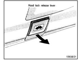
To open the hood, pull the hood lock release lever under the dash. The hood will spring up slightly. In front of the vehicle, press up on the auxiliary catch lever and lift the hood. Then hold the hood open by inserting the support rod into the slot.
