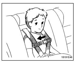
**6. Fasten the shoulder belt clip.** The purpose of the clip is to keep the shoulder belts positioned correctly on the shoulders.
