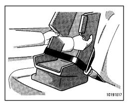
Make sure the seat belt is securely locked. Also make sure the child restraint system is secure by pushing and pulling it in different directions.
