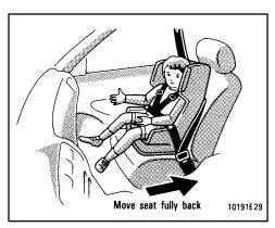
When using a forward-facing child restraint system, move the seat as far back as possible.
