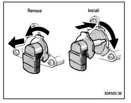
**3. Turn the bulb and remove it. Install the new bulb and install the connector.** To install a bulb, align the tabs of the bulb socket with the cutouts of the mounting hole.
