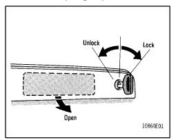
To open the back door from the outside, insert the key and turn it counterclockwise to unlock. Then pull the handle and raise the back door.
