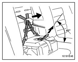
2. While pulling the seat belt release strap in the child seat cushion, pull both shoulder belts together.
