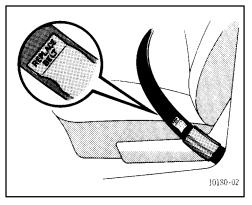
Replace the front seat belt if the warning label under the sleeve can be seen. The warning label, "RE-PLACE BELT", will appear if the belt receives a severe impact or other force.
