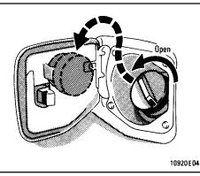
2. To remove the fuel tank cap, turn the cap slowly counterclockwise, then pause slightly before removing it. After removing the cap, hang it on the cap hanger.
