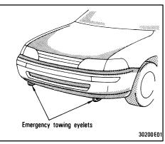
If towing service is not available in an emergency, your vehicle may be temporarily towed by a cable secured to emergency towing eyelets under the front of the vehicle.
