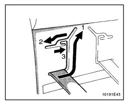
To move the shoulder belts from the lower slot to the upper slot:
