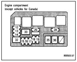
**14. FAN-I/UP 7.5 A:** Multiport fuel injection system/sequential multiport fuel injection system
