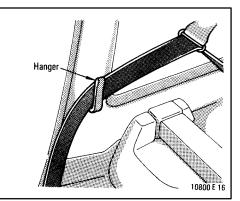
Make sure the shoulder belt passes through the hanger when folding the seatback down.
