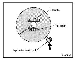
The odometer records the total distance the vehicle has been driven. The trip meter may be set to zero to record the distance on each trip. To reset the trip meter, press the trip meter reset knob.
