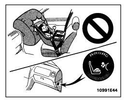
(D)INSTALLATION ON FRONT SEAT— —Vehicles with front passenger airbag
