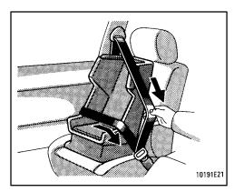
2. Fully extend the shoulder belt to put it in the lock mode.
