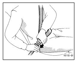
Adjust the seat as needed (front seats only) and sit up straight and well back in the seat. To fasten your belt, pull it out of the retractor and insert the tab into the buckle.
