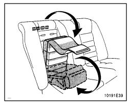
1. Separate the fastener tapes behind the head restraint to separate the head pad from the seatback. Lower the child restraint cushion and fold back the head pad under the child restraint cushion.
