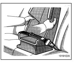
Push and pull the child restraint system in different directions to be sure it is secure.
