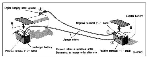
To avoid serious personal injury and damage to your vehicle which might result from battery explosion, acid burns, electrical burns, or damaged electronic components, these instructions must be followed precisely.
