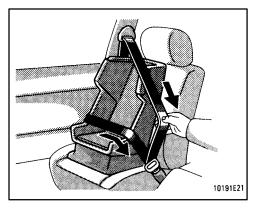
2. Fully extend the shoulder belt to put in the lock mode.
