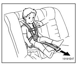
7. Pull the seat belt adjustment strap firmly until the shoulder belts are snugly adjusted around the child's shoulders.
