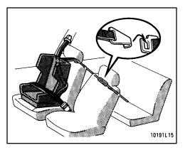
4. If your child restraint system requires the use of a top strap, latch the hook onto the tab of the rear center belt and tighten the top strap.
