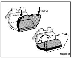
2. Unlock the seatback, and fold it down while pushing the bottom cushion forward.
