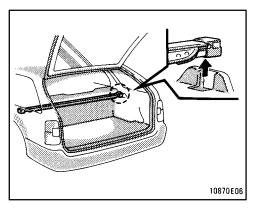
To use the luggage cover, pull it out of the retractor and hook it to the anchors.
