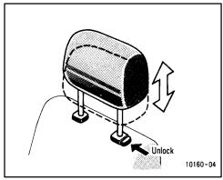
To raise the head restraint, pull it up. To lower it, press the lock release button and push the head restraint down.
