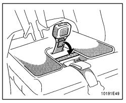
9. To store the built-in child restraint, fasten the shoulder belt clip and return the seat belt buckle using the fastener tapes. Fold up the seat belt adjustment strap in the seat. Then raise the seat cushion and return the head pad by engaging the fastener tapes while pressing the child restraint cushion and head pad firmly.
