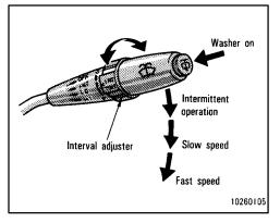
To turn the wipers on, move the lever. To make the washer squirt, push the button on the end of the lever.
