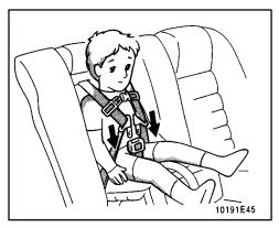
5. Sit the child on the child seat. Place a shoulder belt over each shoulder. Insert the tabs into the buckle.
