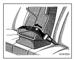
2. Make sure the belt is tight by pulling its free end while you firmly push down the child restraint system.
