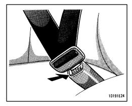
5. To remove the child restraint system, press the buckle-release button and allow the belt to retract. Unhook the top strap.
