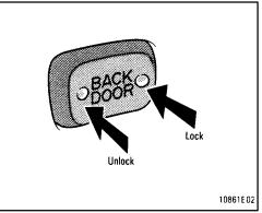
To lock the back door, push the switch on the LOCK side. To unlock the back door, push the switch on the UNLOCK side.
