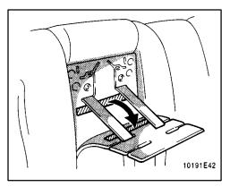
4. Add slack to the shoulder belts by pulling both of them together while pulling the black seat belt release strap (see step 4 for illustrated instruction). Then pull down the seatback part of the removable pad. Determine the proper shoulder belt slot height for your child. Select the slots at or just above the top of the child's shoulders. The child seat pad is attached by fastener tapes.
