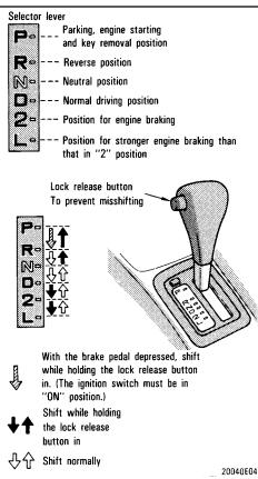
Your automatic transmission has a shift lock system to minimize the possibility of incorrect operation. This means you can only shift out of "P" position when the brake pedal is depressed (with the ignition switch in "ON" position and the lock release button depressed).
