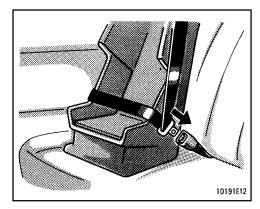
1. Fasten the lap and shoulder belt over the child restraint system following the instructions provided by its manufacturer. Keep the lap portion of the belt tight.
