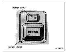
To adjust a power rear view mirror, first push the master switch in "L" (left) or "R" (right) depending on which mirror needs adjusting, then push the control switch in desired direction.
