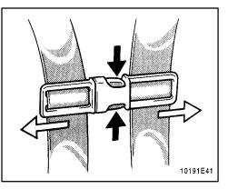
3. Compress the shoulder belt clip to separate the right and left shoulder belts.
