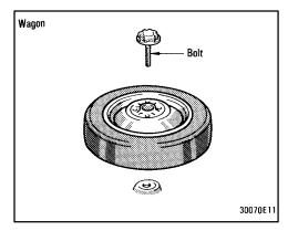
To remove the spare tire, loosen the bolt and remove it.
