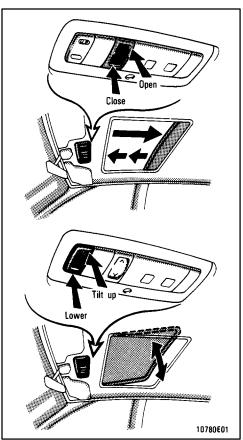
To open the sun roof, push the switch on the "SLIDE" side. Pushing on the opposite side will close it. To tilt up the rear end of the sun roof, push the switch on the "UP" side. Pushing on the opposite side will lower it.
