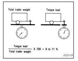
• The trailer cargo load should be distributed so that the tongue load is 9 to 11% of the total trailer weight, not exceeding 68 kg (150 lb.). Never load the trailer with more weight in the back than in the front. About 60% of the trailer load should be in the front half of the trailer and the remaining 40% in the rear.
