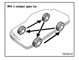
To equalize the wear and help extend tire life, Toyota recommends that you rotate your tires every 12000 km (7500 miles). However, the most appropriate timing for tire rotation may vary according to your driving habits and road surface conditions.
