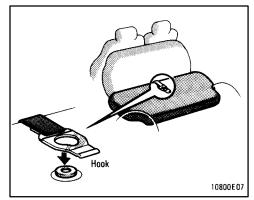
3. After folding the seatback down, hook the strap to the tab on the reverse side of the seatback.
