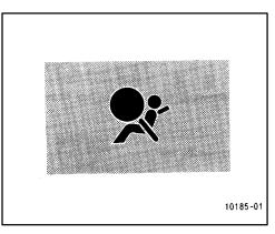
This indicator comes on when the ignition key is turned to the "ACC" or "ON" position. It goes off after about 6 seconds. This means the SRS airbags are operating properly.
