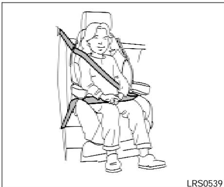
2. Position the booster seat on the seat. Only place it in a front facing direction. Always follow the booster seat manufacturer's instructions.
