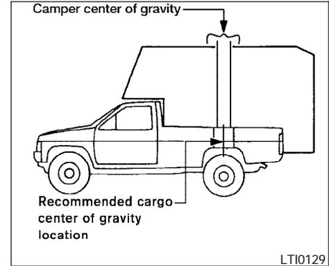
When the truck is used to carry a slide-in camper, the total cargo load of the truck consists of the camper manufacturer's weight figure, plus:
