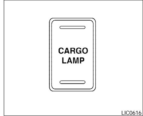
To turn on the cargo lamp, push the switch down to the ON position.
