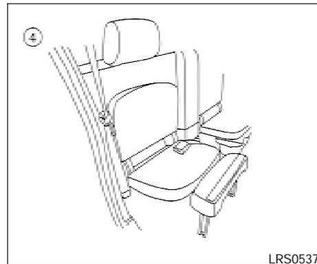
1. To access the jump seat extension ① on the passenger's side jump seat only pull up ② on the extension to unfold it to the open position. Then unfold the two support legs ③ and lower the jump seat to the full open ④ seating position.
