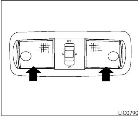
To turn the personal lights on, press the switches. To turn them off, press the switches again.
