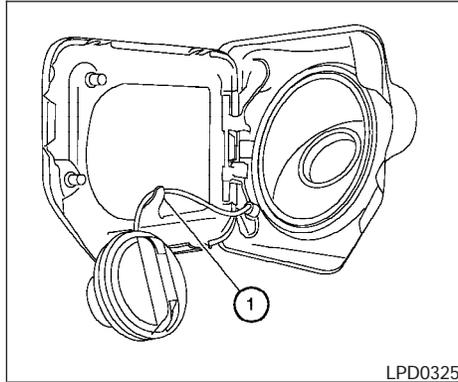
Loop the tether strap around the hook ① while refueling.
