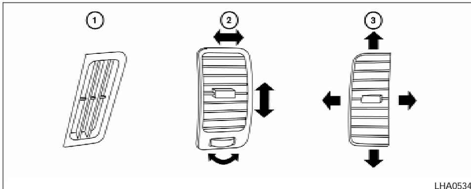
Adjust air flow direction for the driver's and passenger's side windows①, driver and passenger②, or center③ ventilators by moving the ventilator slide and/or ventilator assemblies.
