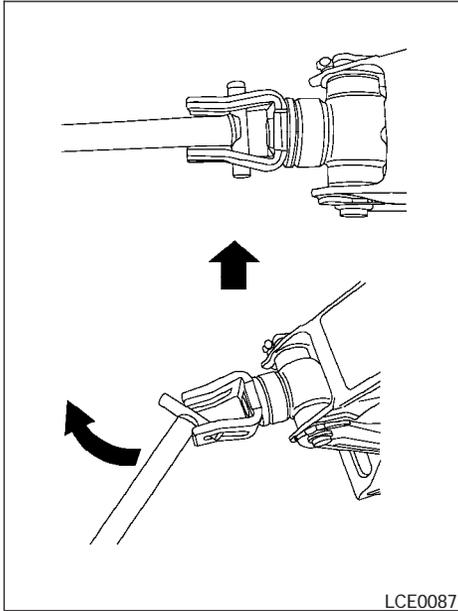
3. Install the assembled jack rod into the jack as shown.
