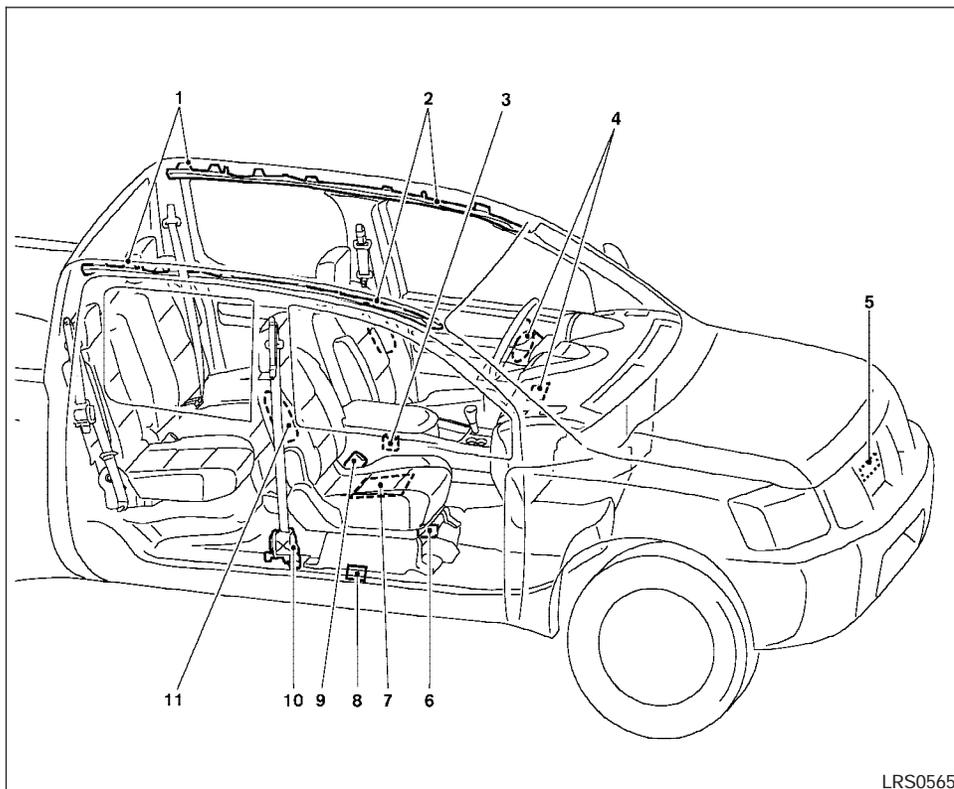
1. SRS curtain side-impact and rollover air bag modules (if so equipped)
