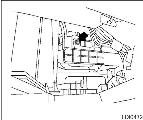
2. Remove the filter cover bolt and remove the filter cover.
