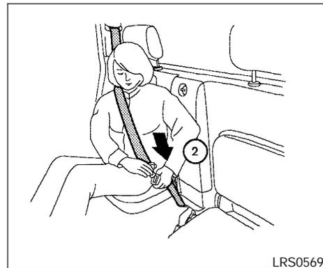
2. Slowly pull the seat belt out of the retractor and insert the tongue into the buckle until you hear and feel the latch engage.
