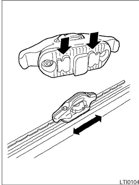
4. Position the cleat so the nubs on the bottom fully seat into the channel detents.
