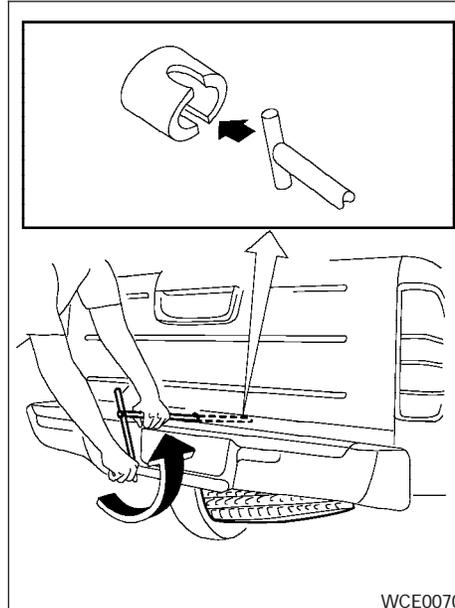
3. Seat the T-shaped end of the jack rod into the T-shaped opening of the spare tire winch. Apply pressure to keep the jack rod engaged in the spare tire winch and turn the jack rod counterclockwise to lower the spare tire.
