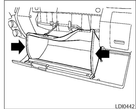
1. Open the glove box and press in on the sides so that it will open completely allowing it to hang by the cord.
