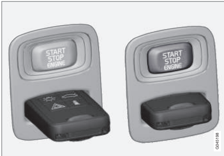
Ignition slot with remote key inserted ( see page 88 for more information on ignition modes)
