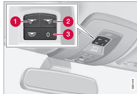
Light switches, front roof lighting
