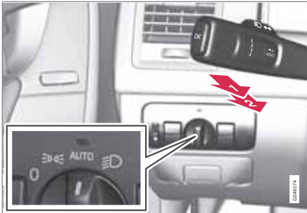
Headlight switch with AUTO and lever
