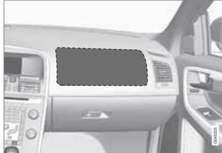
Location of the passenger's side front airbag
