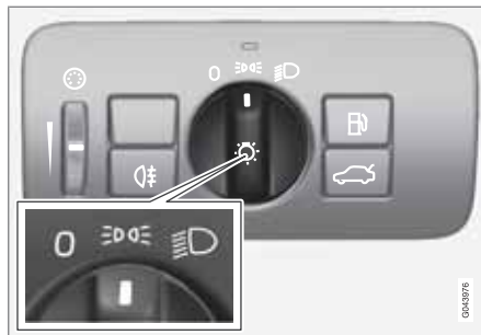
Headlight control in position for parking lights
