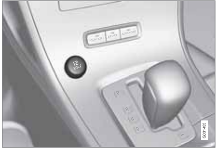
12-volt socket in the front tunnel console
