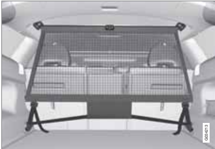
Cargo net mounted in rear position
