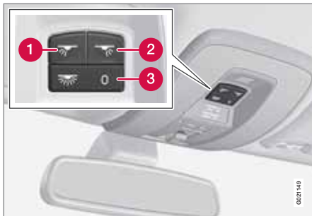
Light switches, front roof lighting
