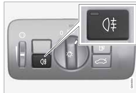
Headlight control in position for parking lights
