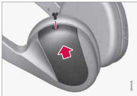
Battery cover and retaining screw
