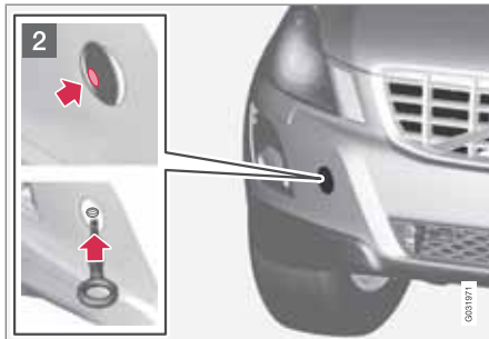
Attaching the towing eyelet
