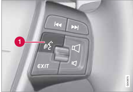
Voice control button (1) on the steering wheel.
