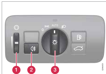
Overview, light switches with AUTO function
