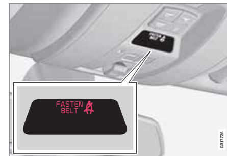
Seat belt reminder light in ceiling console
