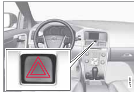
Location of the hazard warning flasher button
