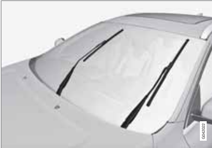
Wiper blades in service position
