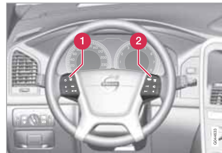
Keypads in the steering wheel
