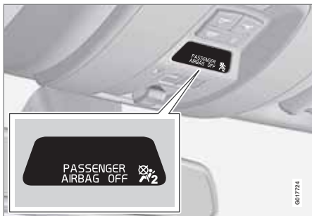
Occupant Weight Sensor (OWS) indicator light
