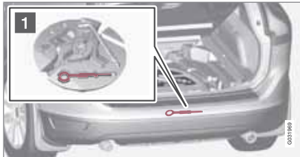
Location of the towing eyelet
