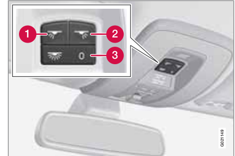
Light switches, front roof lighting
