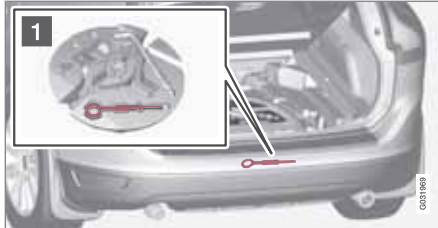
Location of the towing eyelet
