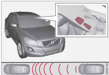
Location of the laser sensor in the windshield
