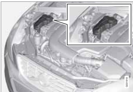
Location of the coolant reservoir
