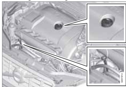
Location of the filler cap and dipstick
