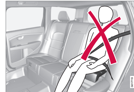
Incorrect seating position: the child's head is above the head restraint and the shoulder belt is not across the collarbone
