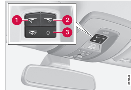
Light switches, front roof lighting
