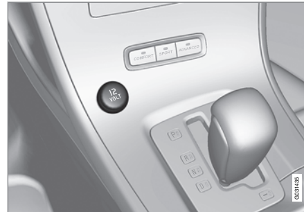
12-volt socket in the front tunnel console
