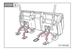
Remove the seat hook covers from the back of the seat cushion, and install them on the seat hooks.
