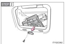
Push the lever for the back door motor, open the back door.
