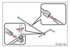
Assemble the jack handle and the jack handle extension bar and tighten the screw.
