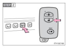
While pressing the desired button ("1", "2" or "3"), press on the wireless remote control until the signal beeps.
