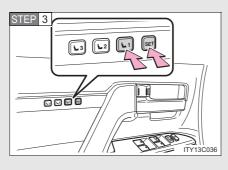
While pressing the "SET" button, or within 3 seconds after the "SET" button is pressed, press and hold button "1", "2" or "3" until the signal beeps.
