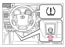
Press and hold the tire pressure warning reset switch until the tire pressure warning light blinks slowly 3 times and the message "TIRE PRESSURE RESET PROCEEDING" appears on the multi-information display.
