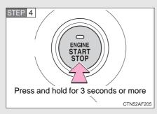
Stop the engine by pressing and holding the "ENGINE START STOP" switch for 3 consecutive seconds or more.
