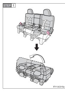
Fold down the seatback while pulling the seatback angle adjustment lever, and swing the whole seat up and forward.
