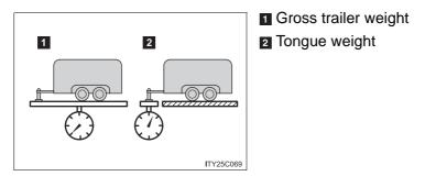
If using a weight distributing hitch when towing, return the front axle to the same weight as before the trailer connection.
