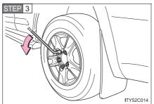
Slightly loosen the wheel nuts (one turn).
