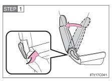
Fold the seatback while pulling the seatback angle lever. Return the seatback and secure it at the first lock position.  $(\rightarrow P. 55)$
