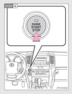
Press the "ENGINE START STOP" switch.
