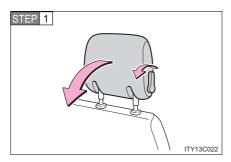
Fold down the head restraints while pulling the head restraint angle lever.
