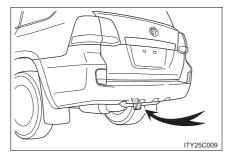
Use the wire harness stored in the rear end under the vehicle body.
