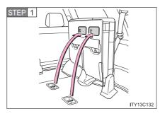
Remove the seat hook covers from the floor and install them into the back of the seat cushion.
