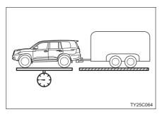
The maximum allowable gross vehicle weight. The gross vehicle weight is the total weight of the vehicle. When towing a trailer, it is the sum of the vehicle weight (including the occupants, cargo and any optional equipment installed on the vehicle) and the tongue weight. When driving
