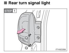
Open the back door and remove the bolts and lamp assembly.
