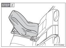
Place the child restraint system on the second or third seat facing the rear of the vehicle.
