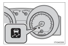
If the vehicle is in danger of slipping, rolling backwards when starting on an incline, or if the rear wheels spin, the slip indicator light flashes to indicate that the VSC/Active TRAC/hill-start assist control systems have been engaged.
