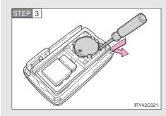
Remove the depleted battery.
