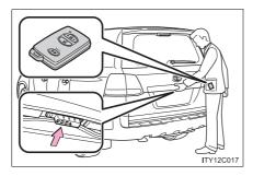
Press the unlock button to unlock the doors.
