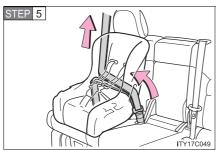
While pushing the child restraint system into the seat, allow the shoulder belt to retract until the child restraint system is securely in place.
