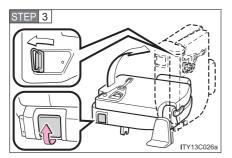
Pull the seat leg lock release levers.
