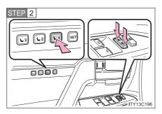
While pressing the desired button ("1", "2", or "3"), press the lock or unlock side on the door lock switch until the signal beeps.
