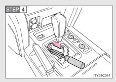
Pry the cover up with a flathead screwdriver or equivalent.
