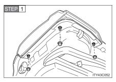
Open the back door and remove the nuts and lamp assembly.
