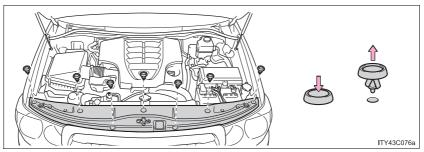
Installing the clips
