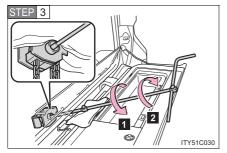
Insert the jack handle extension into the lowering screw.
