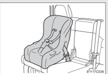
Seat belts equipped with a child restraint locking mechanism (ALR/ELR belts except driver's seat belt) ( $\rightarrow$ P. 72)
