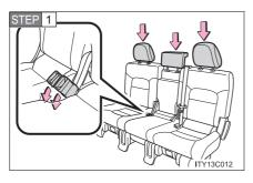
Stow the seat belt buckles and lower the head restraints to the lowest position.
