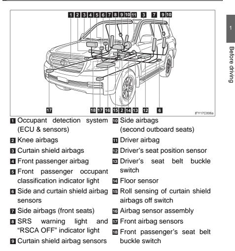
Your vehicle is equipped with ADVANCED AIRBAGS designed based on US motor vehicle safety standards (FMVSS208). The airbag system controls airbag deployment power for the driver and front passenger. The driver airbag system consists of the driver seat's position sensor etc. The front passenger's airbag system consists of the front passenger occupant classification sensor etc.
