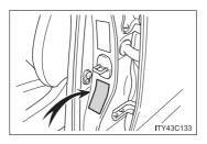
For the GAWR, see the Certification Label. For the maximum load of the tire, see the load limit at maximum cold tire inflation pressure mentioned on the sidewall of the tire. ( $\rightarrow$ P. 575)
