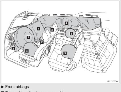
Driver airbag/front passenger airbag
