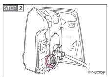
Turn the bulb bases counter-clockwise.
