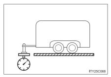
The load placed on the trailer hitch ball. ( $\rightarrow$ P. 242)
