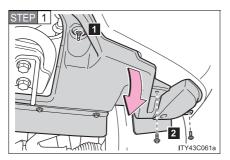
Remove the fender liner bolts, loose the fender liner nut and remove the fender liner.
