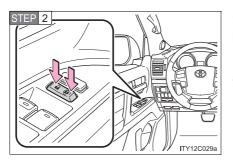
Shift the shift lever to "P" or "N", press and hold the driver's door
