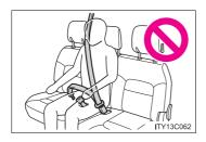
Do not use the third center seat belt with either buckle released. Fastening only one of the buckles may result in death or serious injury in case of sudden braking, sudden swerving or a collision.
