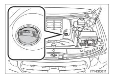
If the oil level is below or near the low level mark, add engine oil of the same type as already in the engine. ( $\rightarrow$ P. 565)
