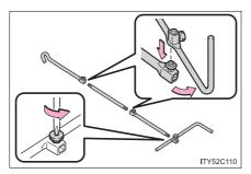
Loosen the bolts and the screw using either the jack handle or a screwdriver.
