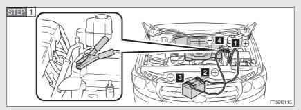
Connecting the jumper cables.
