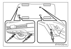
If your Toyota is transported by a flat bed truck, it should be tied down at the locations shown in the illustration. When attaching the hooks to the rear of the vehicle, make sure to attach them to the inside of the vehicle.
