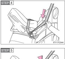
Fully extend the shoulder belt and then allow it to retract slightly in order to activate the ALR lock mode.
