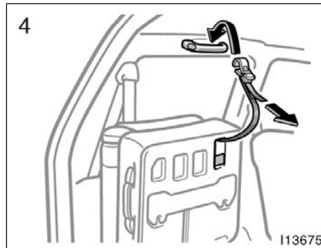
4. Hook the strap. When returning the third seat to its original position, put the holding strap into the hole.
