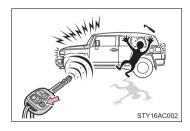
When PANIC button is pushed for longer than about one second, an alarm will sound for about 60 seconds and the vehicle lights will flash to deter any person from trying to break into or damage your vehicle.
