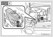
Inspect the amount of engine coolant by checking if the reservoir level is between the F (Full) and L (Low) lines.
