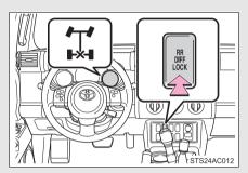
Press the RR DIFF LOCK switch to lock the rear differential.
