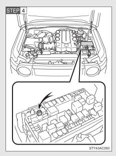
Remove the fuse with the pullout tool.
