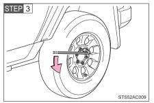
Slightly loosen the wheel nuts (one turn).
