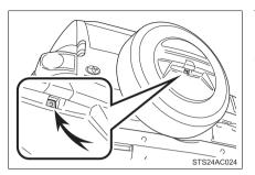
The camera for the rear view monitor system is located to the spare wheel cover.
