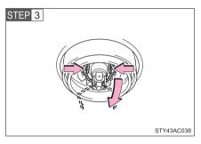
Release the bulb retaining spring.
