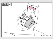
Stop the engine by turning the engine switch to the ACC position.
