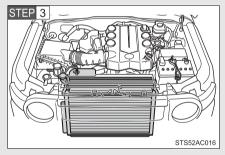
After the engine has cooled down sufficiently, inspect the radiator core (radiator), hoses, etc. for any leaks.
