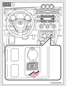
Open the cover and connect an iPod using an iPod cable.
