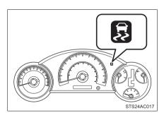
If the rear wheels spin, the slip indicator flashes to indicate that the AUTO LSD system has controlled the spinning of the rear wheels.
