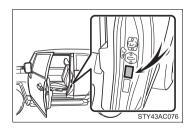
For the GAWR, see the Certification Label. For the maximum load of the tire, see the load limit at maximum cold tire inflation pressure mentioned on the sidewall of the tire. ( $\rightarrow$ P. 524)
