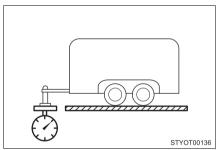
The load placed on the trailer hitch ball. ( $\rightarrow$ P. 220)
