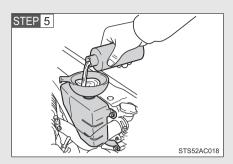
Add engine coolant if necessary.
