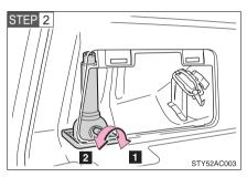
Loosen and remove the jack.
