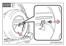
Remove the bolt which fixes the spare wheel cover using the wrench in the tool bag  $(\rightarrow P. 482)$ .
