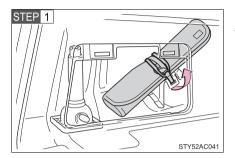
Remove the cover and loosen the strap.
