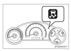
If the vehicle is in danger of slipping, or if the rear wheels (2WD models) or any of the drive wheels (4WD models) spins, the slip indicator flashes to indicate that TRAC (TRC)/VSC have been engaged.
