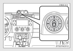
The compass points north for about 3 seconds after the engine switch is turned to the ON position, and then indicates the actual direction the vehicle facing.
