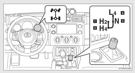
The four-wheel drive indicator comes on when the H4, N or L4 mode is selected.
