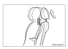
When the occupant's lower back presses against the seatback during a rear-end collision, the head restraint moves slightly forward and upward to help reduce the risk of whiplash on the seat occupant.
