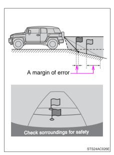
The distance guide lines will appear to be farther from the vehicle than the actual distance. Because of this, objects will appear to be closer than they actually are. In the same way, there will be a margin of error between the guide lines and the actual distance/course on the road.
