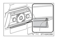
Install the rubber inside the panel as shown in the illustration.
