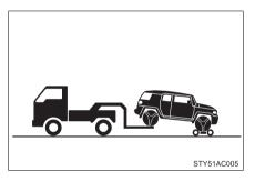
Vehicles with an automatic transmission: When not using a towing dolly, turn the engine switch to the ACC position, shift the shift lever to N and shift the frontwheel drive control lever in H2.
