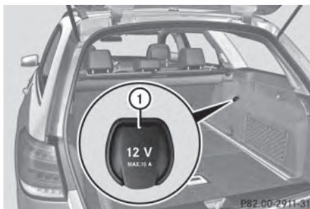
Power socket in the cargo compartment (Wagon)
