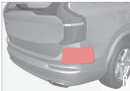
Location of rear radar sensors. Keep the marked area clean (on both the left and right sides of the vehicle).
