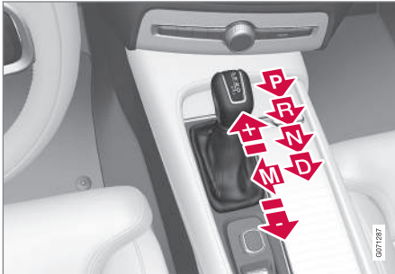
Large gear selector and gear selector positions overview.
