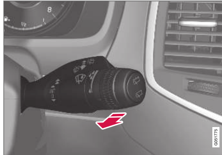
Washing function, right-hand steering wheel lever.
