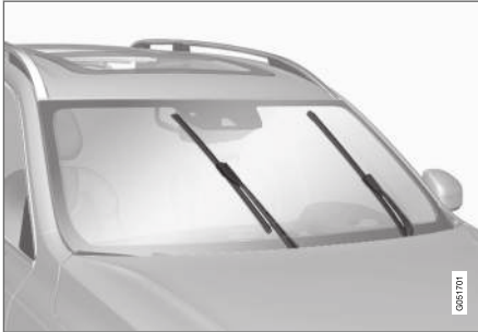
Windshield wipers in the service position.
