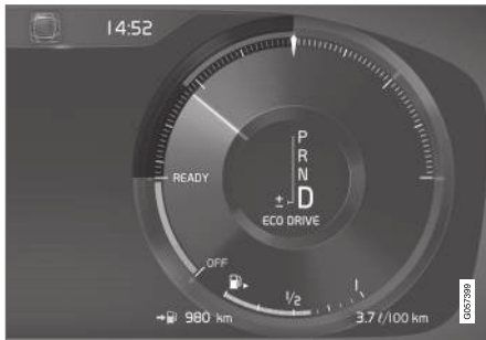
Eco gauge in 12" instrument panel*.
