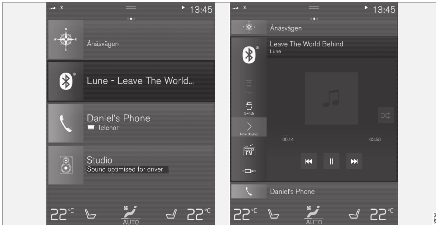
Standard mode and expanded mode of a tile in the center display.
