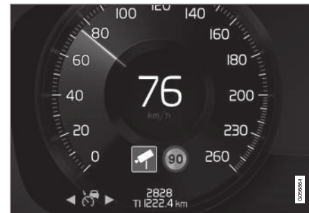
Speed camera information in the instrument panel 100 .
