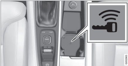
Back-up reader in the tunnel console
