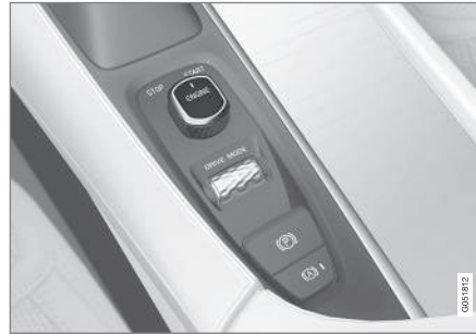
Start knob in the tunnel console between the front seats (generic illustration)
