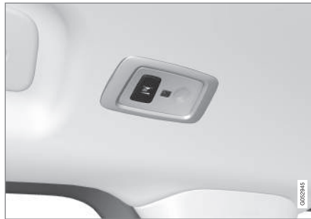
Rear reading light: second row of seats in models with a laminated panoramic roof*
