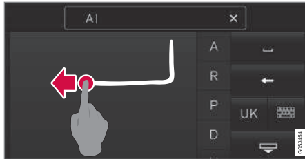
Create a new line by drawing above the characters as shown in the illustration
