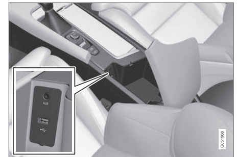
USB socket in the tunnel console
