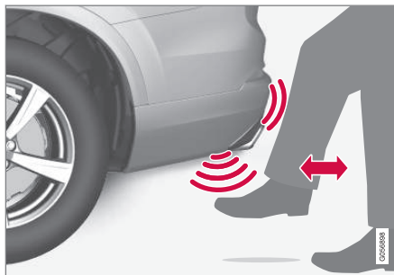
Kicking motion under the sensor's activation area
