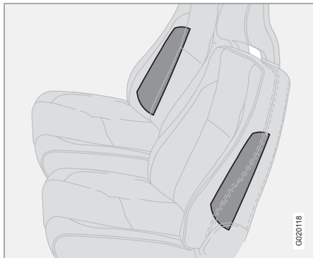
Location of the side impact (SIPS) airbag
