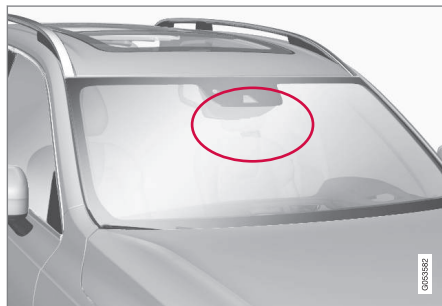
Radar unit location.
