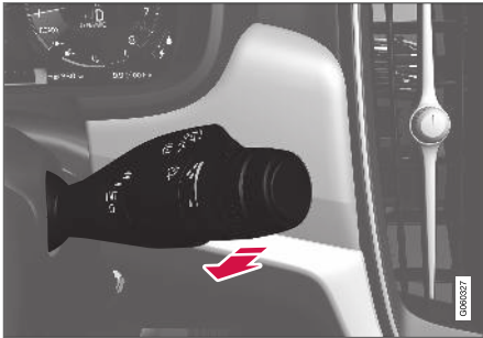
Washing function, right-hand stalk switch.
