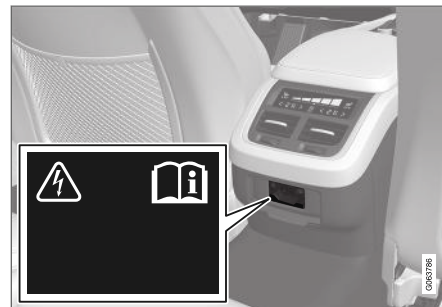
Electrical socket in the tunnel console, rear seat.
