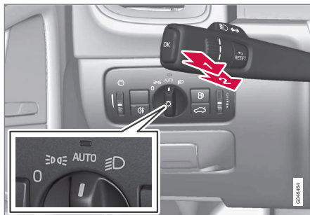
Stalk switch and knob for headlamp control.
