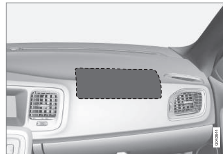
Location of the front passenger airbag in a left-hand drive car.
