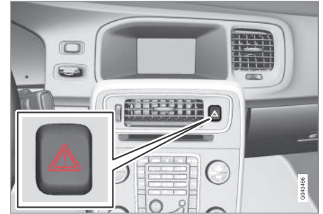
Button for hazard warning flashers.
