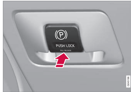
Parking brake control - apply.
