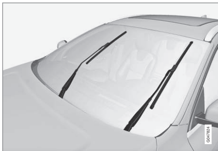
Wiper blades in service position.
