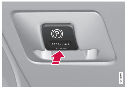
Parking brake control - apply.
