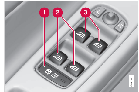
Driver's door control panel.
