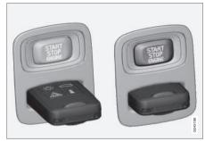
Ignition switch with remote control key extracted/inserted.
