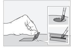
Before work is begun, the car must be clean and dry and at a temperature above 15  $^\circ C.$
