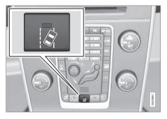
Press the button in the centre console to activate or deactivate the function. The function is switched on if one lamp is illuminated in the button.
