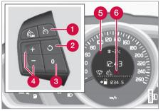
The steering wheel buttons and combined instrument panel in cars **with** speed limiter<sup>4</sup>.
