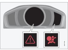
Warning triangle and warning symbol for the airbag system in the digital combined instrument panel.
