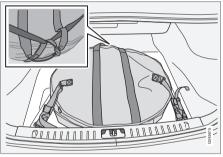
Cars with two load retaining eyelets.
