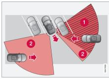
In an angled parking slot CTA can be completely "blind" on one side.
