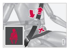
It is important that the seatbelt lies against the body so it can provide maximum protection. Do not lean the backrest too far back. The seatbelt is designed to protect in a normal seating position.
