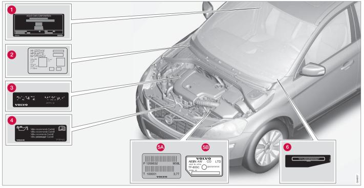
Knowing the car's type designation, vehicle identification and engine numbers can facilitate all contact with an authorised Volvo dealer regarding the car and when ordering spare parts and accessories.
