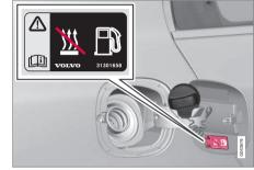
The fuel filler cap can be attached onto the flap.
