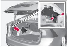
The bulbs in the rear light cluster are replaced from inside the cargo area (not the LED lamps).
