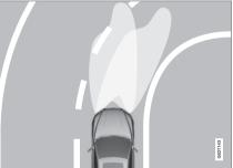
Headlamp pattern with function deactivated (left) and activated (right) respectively.
