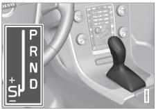
D: Automatic gear positions. +/-: Manual gear positions. **S**<sup>8</sup>: Sport mode\*.
