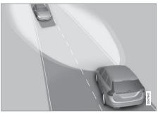
Dipped beam directly toward oncoming vehicles, but continued main beam on both sides of the vehicle.
