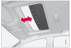
One long press on the lock button closes the sunroof and all the windows, see Remote control key - functions (p. 146) and Locking/ unlocking - from the inside (p. 160). The doors and the boot lid are locked. To interrupt closing, press the lock button again.
