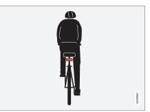
Optimum examples of what the system interprets as a cyclist - with clear body and bicycle contours, directly from behind and in the car's centre line.
