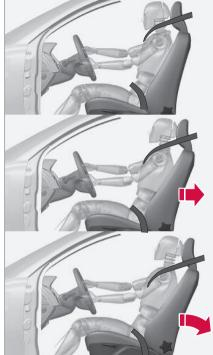
The WHIPS system is actuated by a rear-end collision, where the angle and speed of the collision, and the nature of the colliding vehicle all have an influence.
