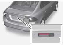
Rubber plate with electrical contact.
