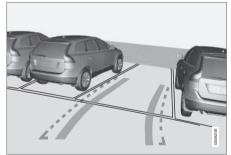
Examples of how the park assist lines can be displayed for the driver.
