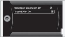
The driver can opt to receive a warning when the applicable speed limit is exceeded by 5 km/h or more. This warning is given by the symbol showing the applicable maximum speed temporarily flashing when this speed is exceeded. The function can be activated/ deactivated in the menu system MY CAR. For a description of the menu system, see MY CAR (p. 99).
