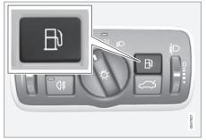
Open the fuel filler flap using the button on the lighting panel - the flap opens when the button is released.
