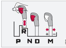
The gear selector can be moved forward and back freely between **N** and **D**. Other positions are locked with a latch that is released with the inhibitor button on the gear selector.
