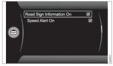
The combined instrument panel's speed symbol display can be disabled. The function can be activated/deactivated in the menu system MY CAR. For a description of the menu svstem, see MY CAR (p. 99).
