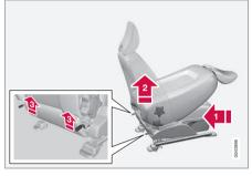
The passenger seat backrest can be folded forward to make room for long loads.
