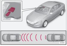
Laser sensor transmitter and receiver window<sup>13</sup>.
