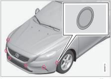
The PAP sensors are located in the bumpers  $^{25}$  - 6 front and 4 rear.
