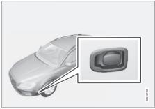
Electrical input to the engine block heater.
