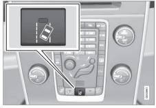
LDW is engaged or disengaged using a button on the centre console. An indicator lamp in the button illuminates when the function is switched on.
