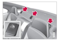
For cars with folding head restraints on the outside seats, the head restraints should be folded to facilitate installation.
