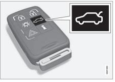
The alarm for the tailgate can be disarmed<sup>\*</sup> and the tailgate unlocked on its own by using the remote control key's 🖂 button.
