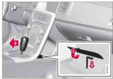
If the car cannot be driven, e.g. due to a flat battery, the gear selector must be moved from the **P** position so that the car can be moved.
