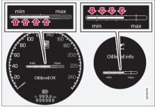
The figures 1-4 represent filling level. Do not fill more oil if filling level (3) or (4) is shown. Recommended filling level is 4. Message and graph in the display. The left-hand display shows the digital combined instrument panel and the righthand the analogue.
