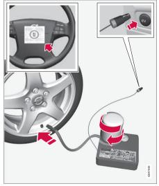
For information on the function of the parts, see Emergency puncture repair kit - overview (p. 329). 1. Detach the label for maximum permitted speed (which is fitted on one side of the compressor) and affix it to the steering wheel.
