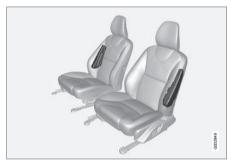
The SIPS bag system consists of two main components, side airbag and sensors. The side airbags are located in the front seat backrests.
