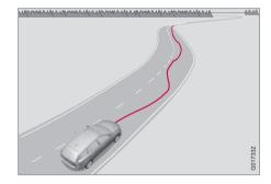
A camera detects the side markings painted on the carriageway and compares the section of the road with the driver's steering wheel movements. The driver is alerted if the vehicle does not follow the carriageway evenly.
