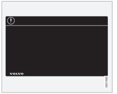
White ISO symbols and white text/image on black or blue warning field and message field. Used to indicate the presence of danger which, if the warning is ignored, may result in damage to property. White ISO symbols and white text/image on black message field.
