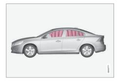
Inflatable curtain IC (Inflatable Curtain) is part of the SIPS system (p. 31) and the airbag system (p. 28). It is fitted in the headlining along both sides of the roof and protects the car's occupants sitting in the outer seats. A sufficiently violent collision trips the sensors and the inflatable curtain is inflated.
