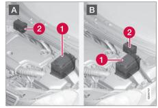
A: Left-hand drive car. B: Right-hand drive car. (1) Starter battery<sup>14</sup> (2) Support battery.
