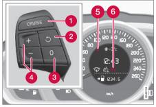
The steering wheel buttons and combined instrument panel in cars **without** speed limiter<sup>4</sup>.
