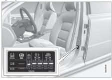
The tyre pressure label on the driver's side door pillar (between frame and rear door) shows which pressures the tyres should have at different loads and speed conditions. This is also specified in the tyre pressure table, see Tyres - approved tyre pressures (p. 399).
