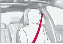
Correctly fitted seatbelt.
