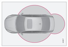
The red rings in the above figure indicate the range covered by the system's antennas.
