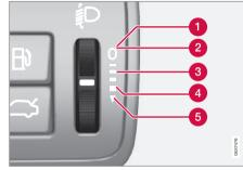
Thumbwheel positions for different load cases.
