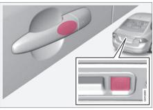
The touch-sensitive area on the outer door handles and a rubberised button next to the boot lid's rubberised pressure plate.
