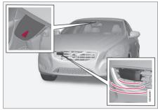
Camera and radar sensor<sup>18</sup>.
