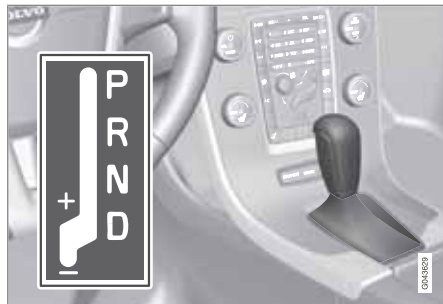
D: Automatic gear positions. +/-: Manual gear positions.
