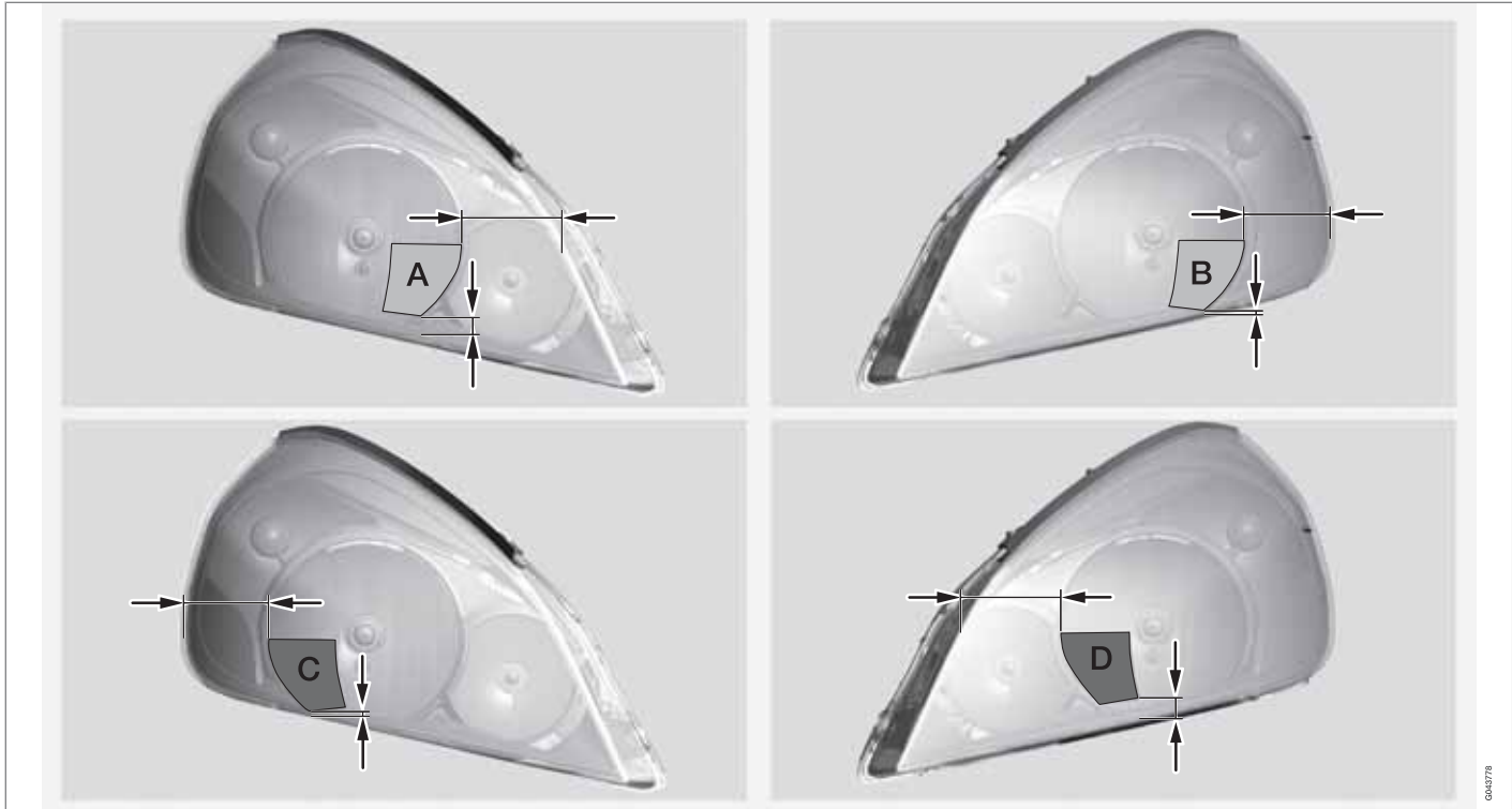
Upper row: left-hand drive cars, templates A and B. Lower row: right-hand drive cars, templates C and D.
