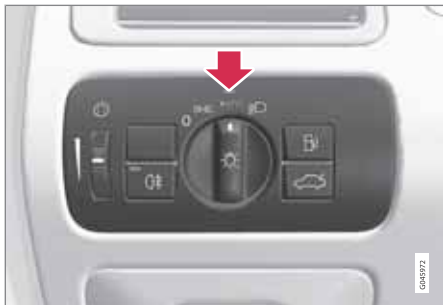
Light switch in position AUTO .
