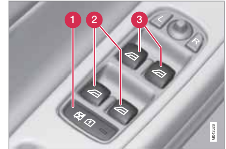
Driver's door control panel.
