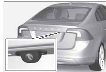
Camera location next to the opening handle.
