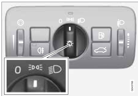
Headlamp control in position for position/parking lamps.
