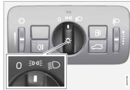
Headlamp control in position for position/parking lamps.
