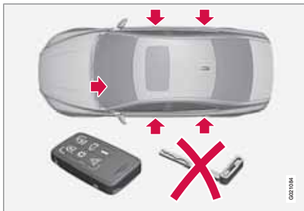
Active locks for remote control key, without key blade and privacy locking activated .
