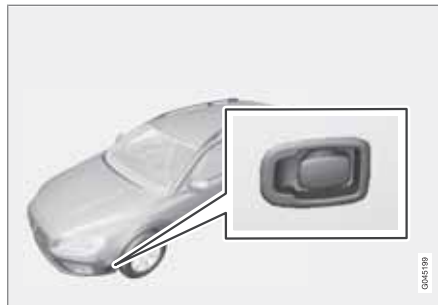
Electrical input to the engine block heater.
